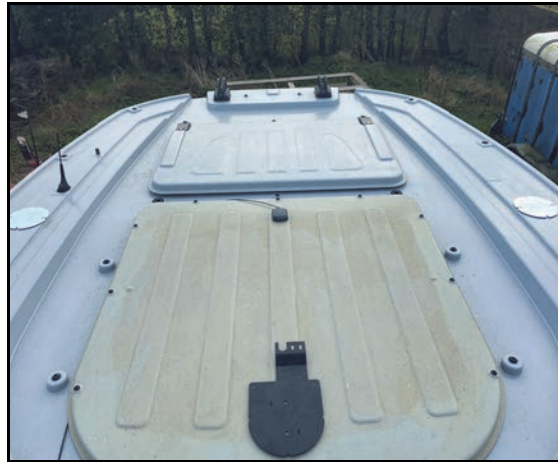
FIGURE 15. GNSS Patch Antenna and Two GPRS/UMTS Antennas
