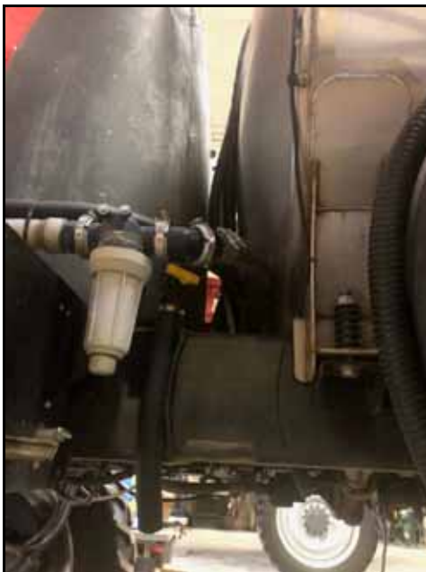
FIGURE 10. Return Hose Routing
