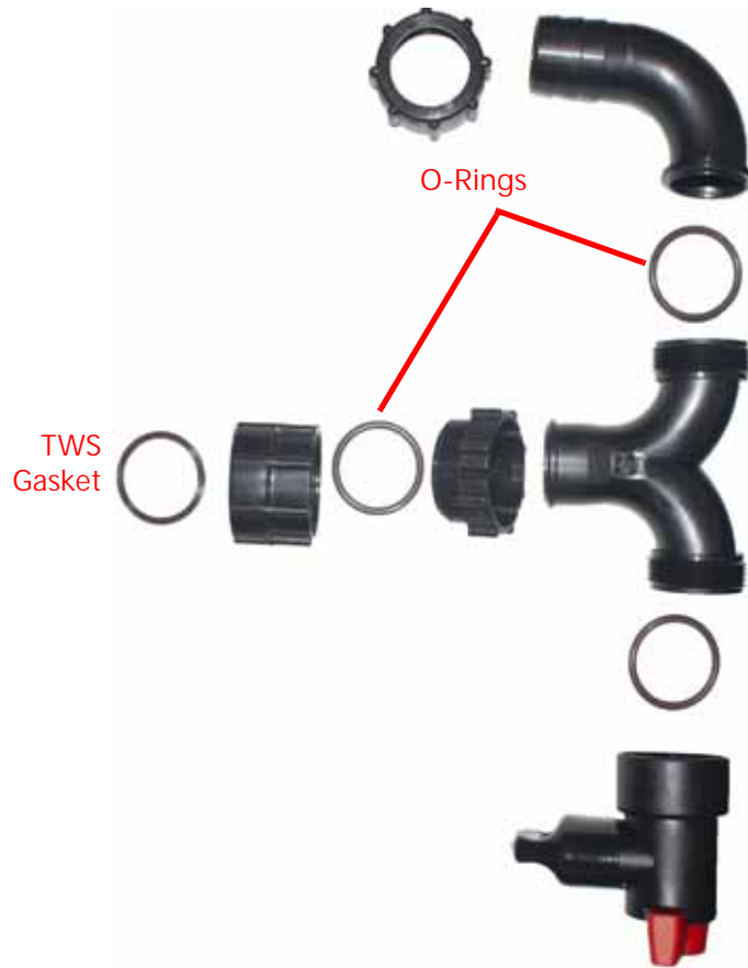
FIGURE 15. Assembly of End Fittings
