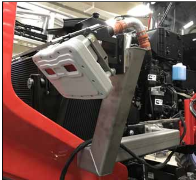
FIGURE 9. Camera Assembly Installed
