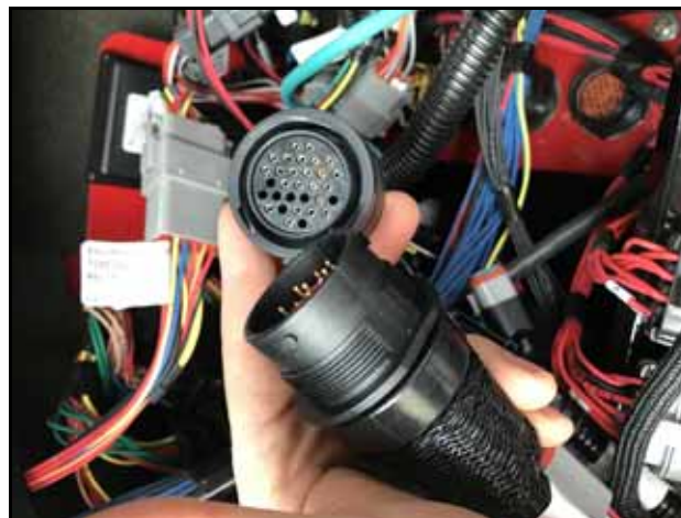
FIGURE 11. Mating Cable Connected to C9 Cable Connector
