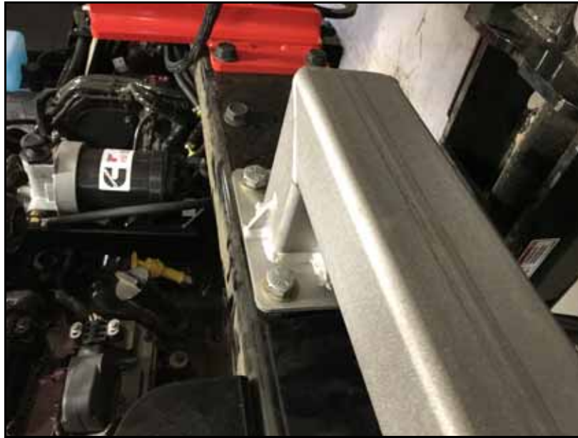
FIGURE 2. VSN Weldment Bracket Mounted to Frame
