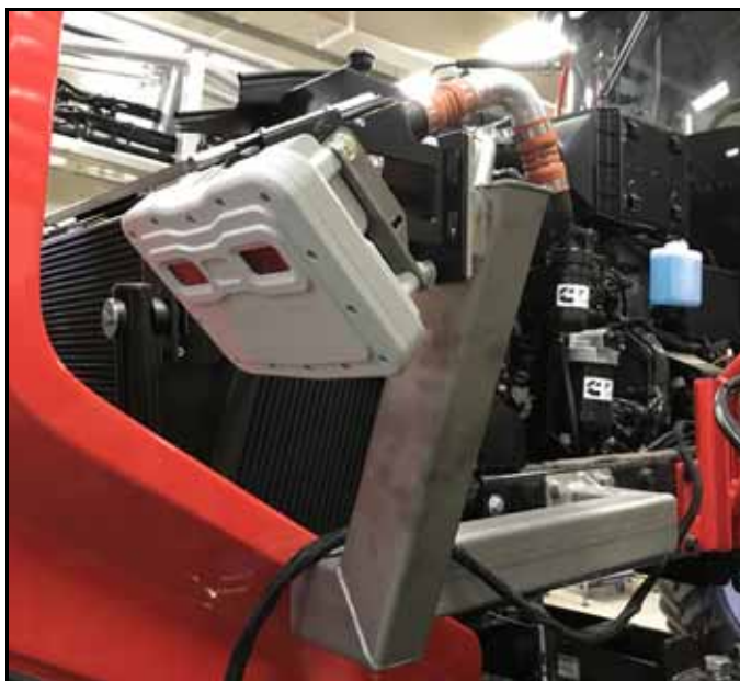
FIGURE 6. Installed Camera Assembly
