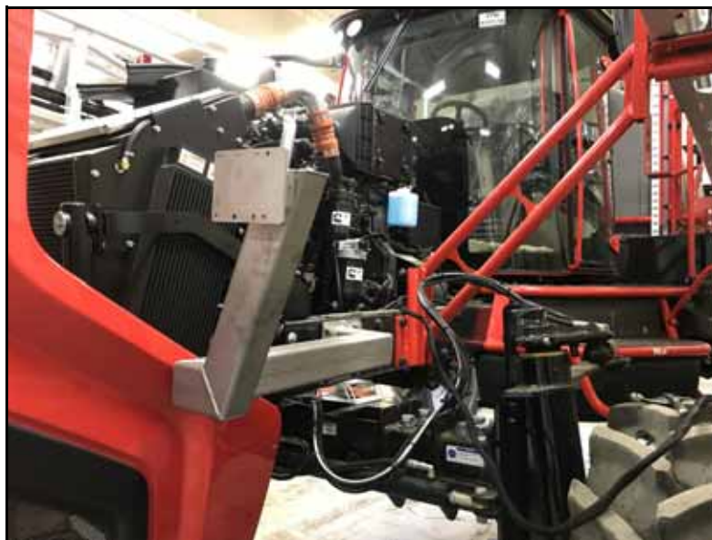
FIGURE 3. VSN Weldment Bracket Level with Frame
