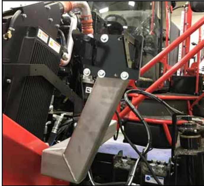
FIGURE 4. Bracket Mounted to the VSN Weldment
