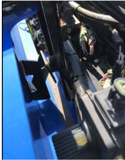
FIGURE 3. Rubber Bumper Installed on Installed Bracket with Front Trim Secured
