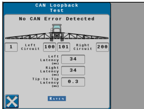
FIGURE 6. NCV Communication Test No CAN Error Detected
