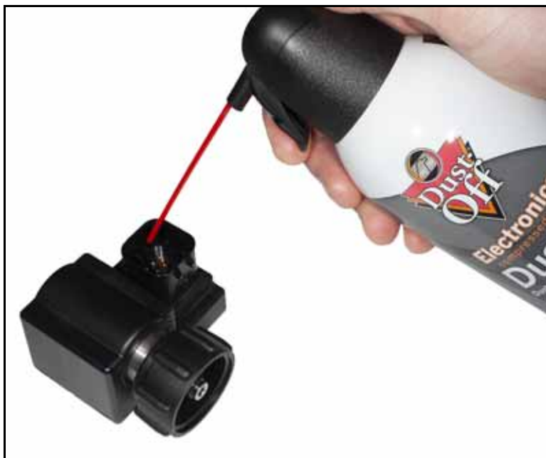
FIGURE 3. Compressed Air Used to Dry Connector
