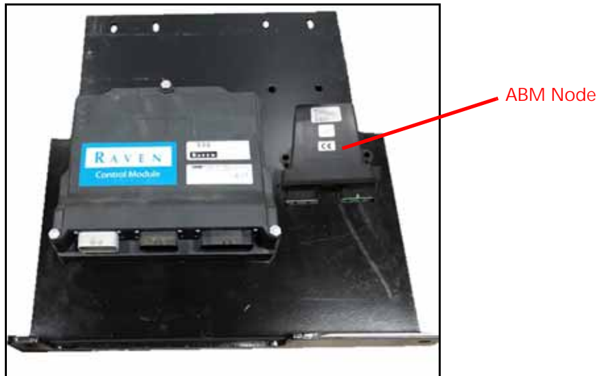
FIGURE 2. REM and ABM Node Mounted
