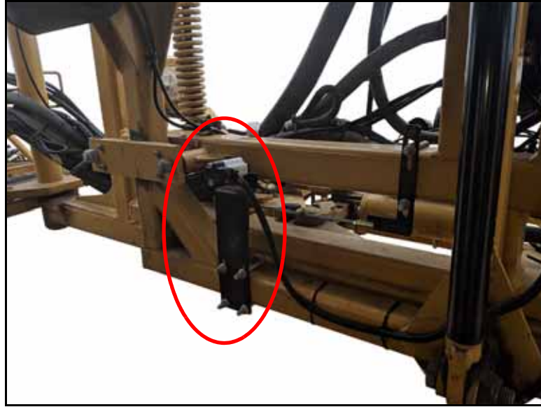
FIGURE 13. Rotary Sensor Installation Location
