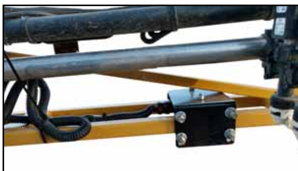
FIGURE 3. Inner Boom Sensor Installed
