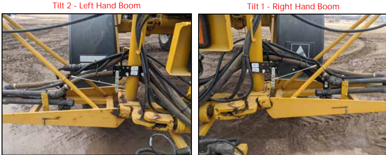
FIGURE 19. Tilt Sensor Installed - Left Hand Boom and Right Hand Boom
