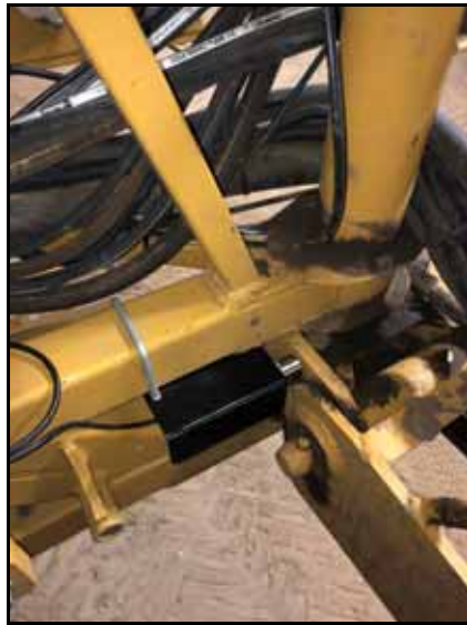
FIGURE 11. Boom Proximity Sensor Bracket
