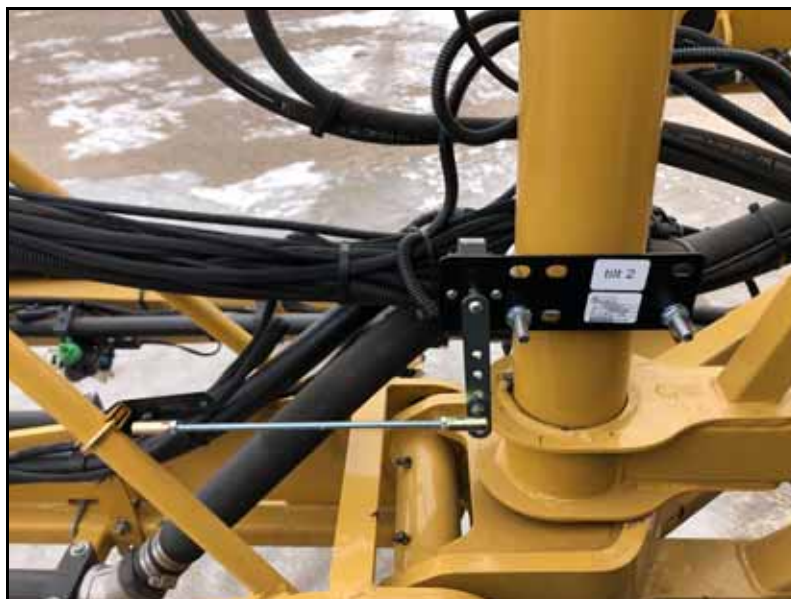
FIGURE 12. Tilt Sensor Installed - Right Hand Boom
