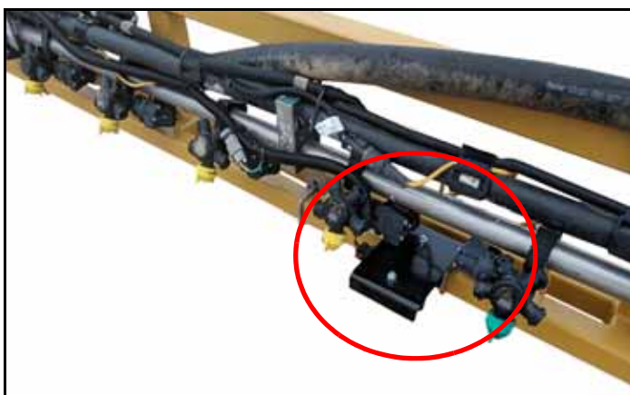
FIGURE 2. Boom Sensor Installed Near End of Boom
