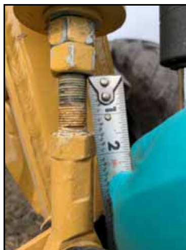
FIGURE 14. Jam Nuts with a Distance of 1.5in
