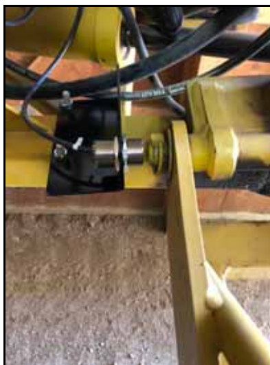
FIGURE 18. Boom Proximity Sensor Bracket
