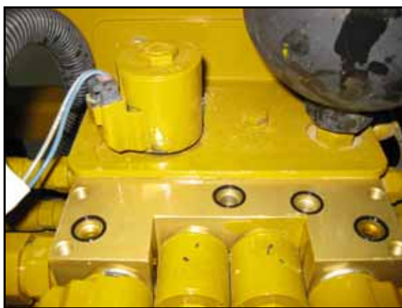
FIGURE 2. O-Rings Placed on the Machine Hydraulic Valve
