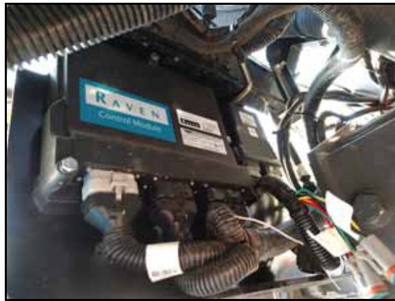
FIGURE 5. AutoBoom Cable Connected to Node
