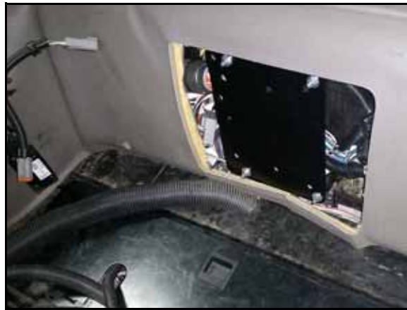
FIGURE 13. HDU Mounting Bracket Installed
