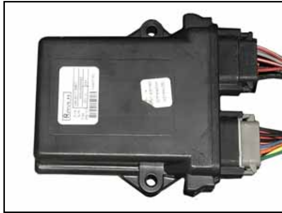
FIGURE 3. HDU Harness Cable Installed on HDU
