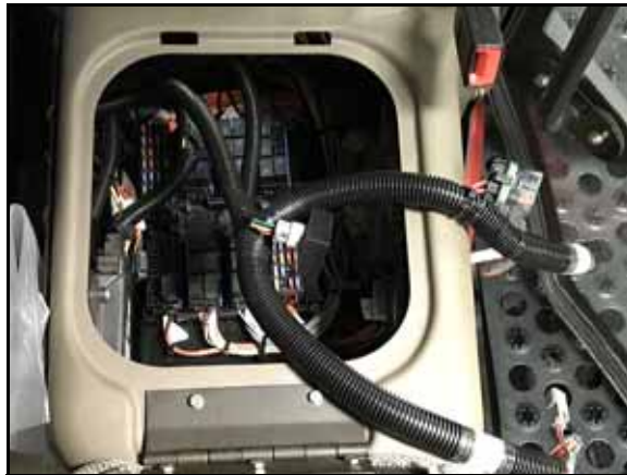
FIGURE 5. SC1 HDU Harness in Instructional Seat Compartment
