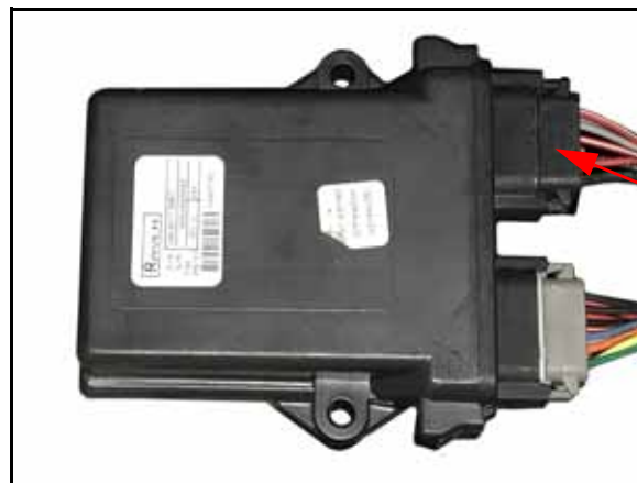
FIGURE 13. SC1 to Bulkhead Cable Installed on HDU
