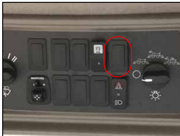
FIGURE 11. Master Switch Installation Location
