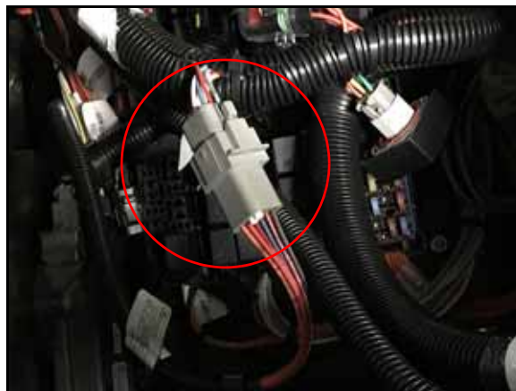
FIGURE 9. HDU Harness Cable Connection
