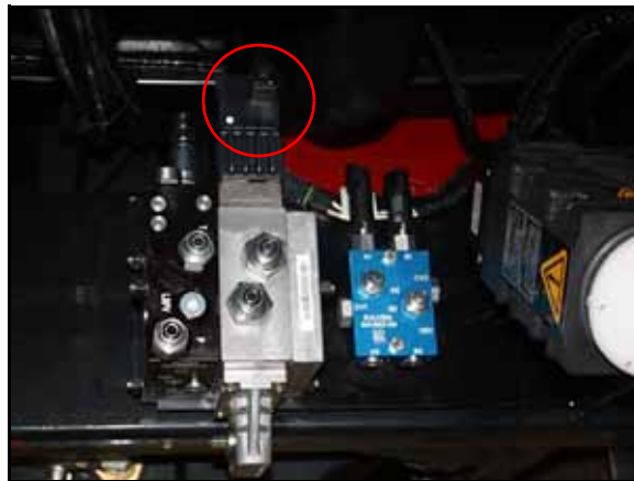
FIGURE 16. VALVE Harness Cable Installation Location
