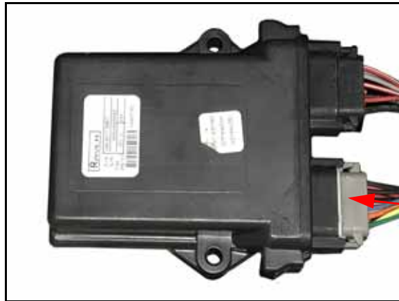
FIGURE 7. SC1 HDU Harness Cable Installed on HDU
