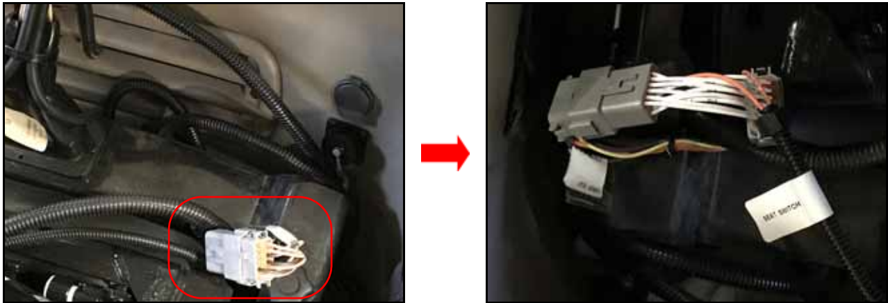
FIGURE 11. Seat Switch Harness Connections
