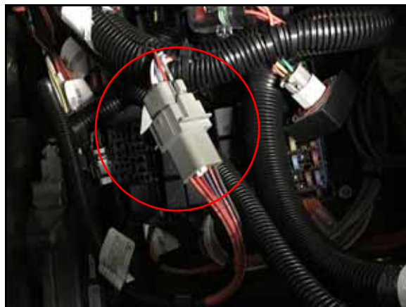
FIGURE 10. HDU Harness Cable Connection
