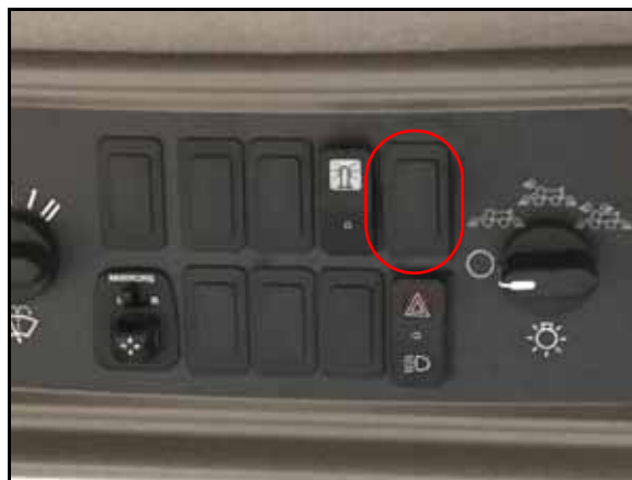
FIGURE 12. Master Switch Installation Location
