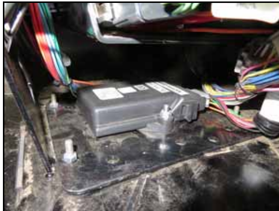
FIGURE 3. Node and Bracket Secured to Floor Studs
