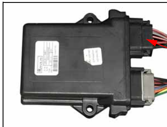
FIGURE 14. SC1 to Bulkhead Cable Installed on HDU
