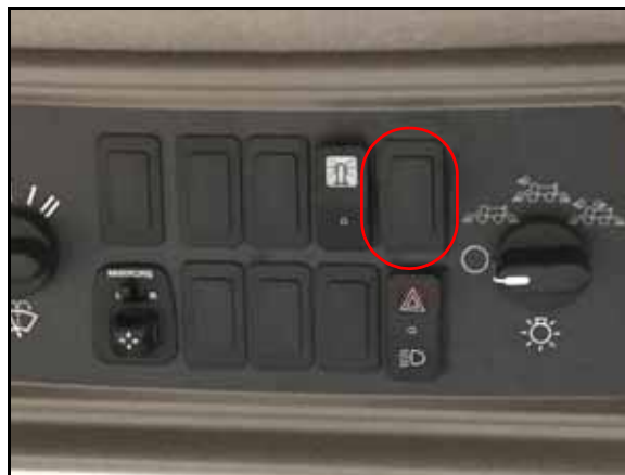
FIGURE 8. Master Switch Installation Location
