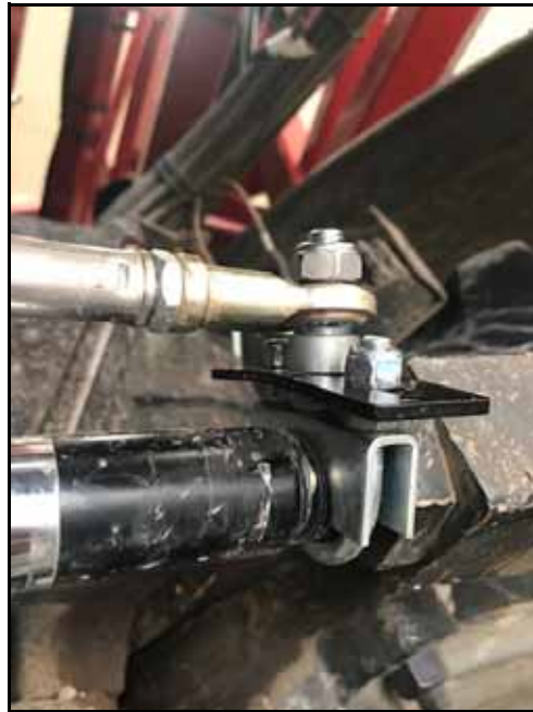
FIGURE 3. Small WAS Mounting Bracket Installed on Rod-End of Steering Cylinder
