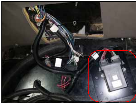
FIGURE 10. HDU Installed on HDU Mounting Bracket
