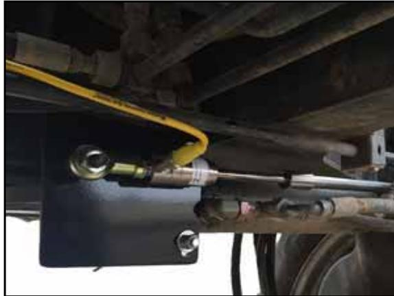
4. Connect the WAS connector to the base-end of the installed WAS (P/N 416-0001-052).
