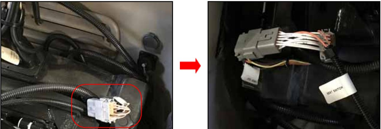
2. Locate and disconnect the machine's seat switch harness connections.
