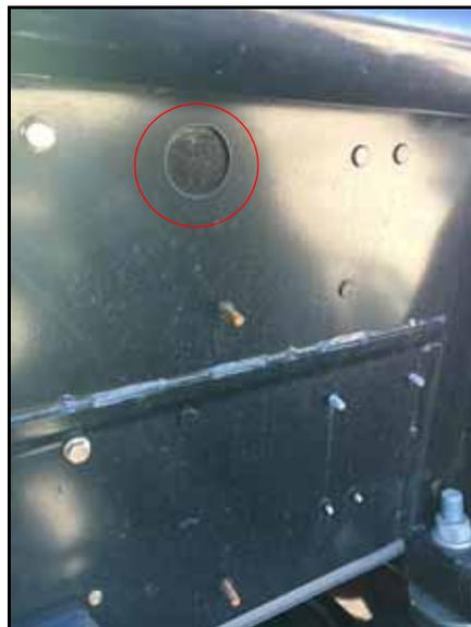
2. Locate the open bulkhead port at the rear of the cab.
