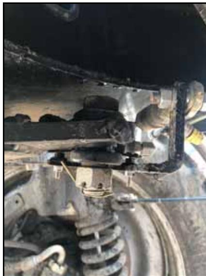
13. Insert an M10 x 1.5 x 35 hex bolt (P/N 311-0070-025) through the back of the WAS base end mounting bracket.
