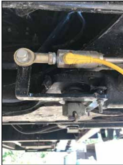
16. Tighten the M10 universal ball mounts and M10 jam nuts to each other on the WAS assembly to ensure they are installed securely.
