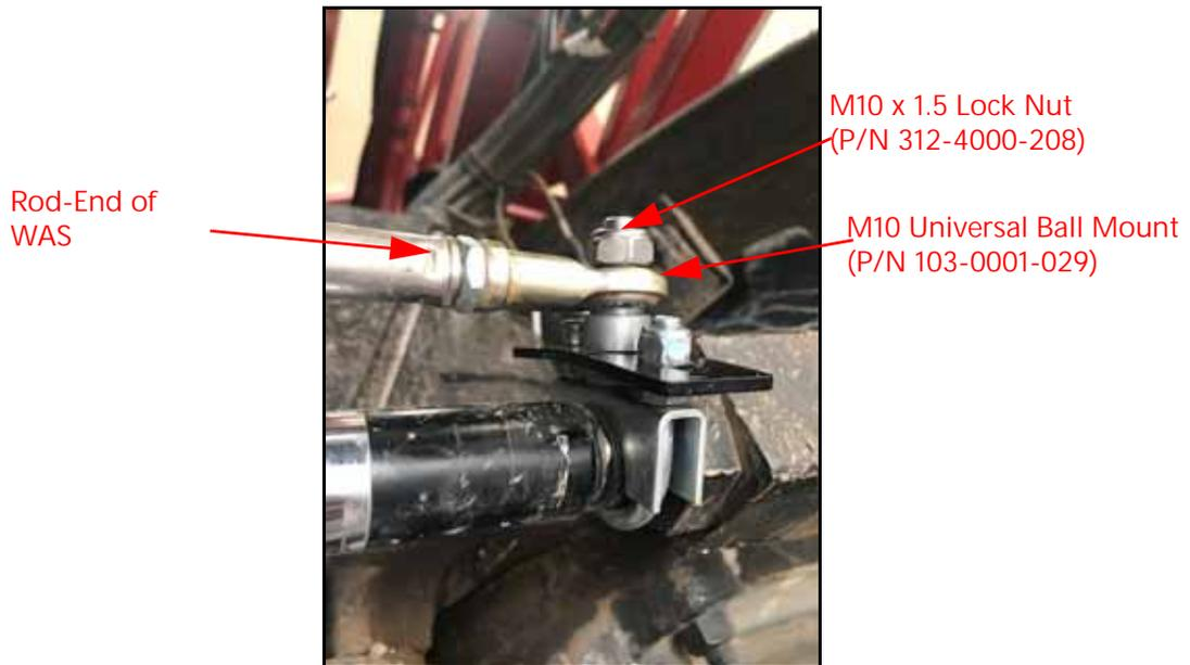
12. Install the ball mount on the rod-end of the WAS assembly on the installed hex bolt and secure it using an M10 x 1.5 lock nut.
