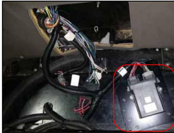
1. Install the HDU (P/N 063-0173-887) on the HDU mounting bracket (P/N 107-0172-543) using two 1/4"-20 flanged lock nuts (P/N 312-1001-168).
