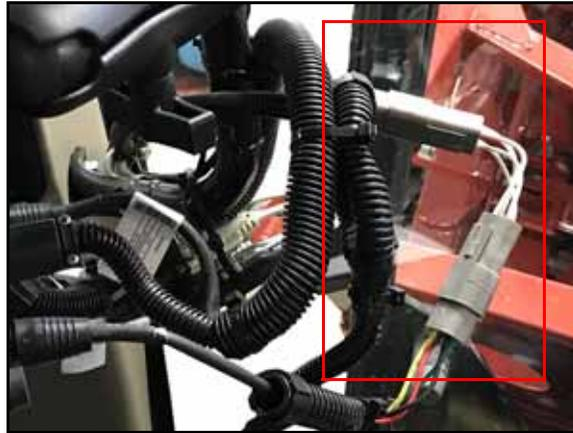
1. Remove the terminator from the 4-pin connector next to the Viper 4 connection of the HDU harness cable (P/N 115-4010-185).
