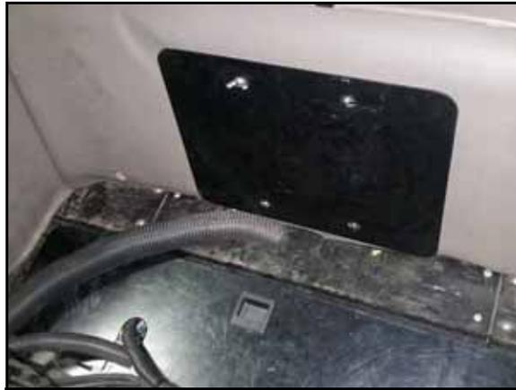
1. Locate and remove the wall panel behind the operator's seat.
