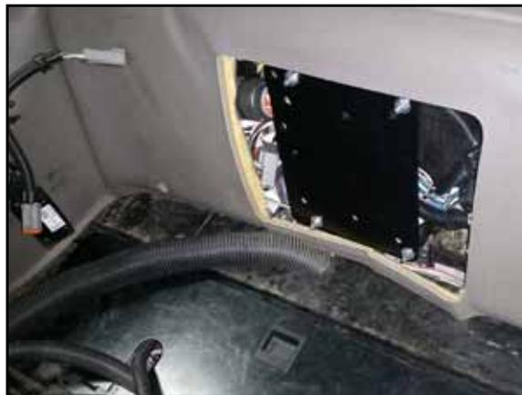
2. Secure the HDU mounting bracket in the access panel so that the HDU faces the cab wall using the existing mounting studs and four M6 flanged lock nuts (P/N 312-4000-216).
