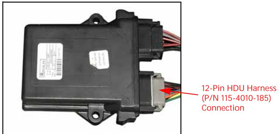
2. Connect the gray 12-pin connector of the SC1 HDU harness cable to the mating port of the HDU (P/N 063-0173-887).
