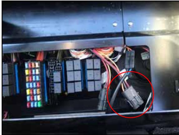
3. Connect the machine's X-024M GPS POWER PORT connector (located in the fuse panel behind the operator's seat) to the mating connector on the power adapter cable (P/N 115-0172-467).
