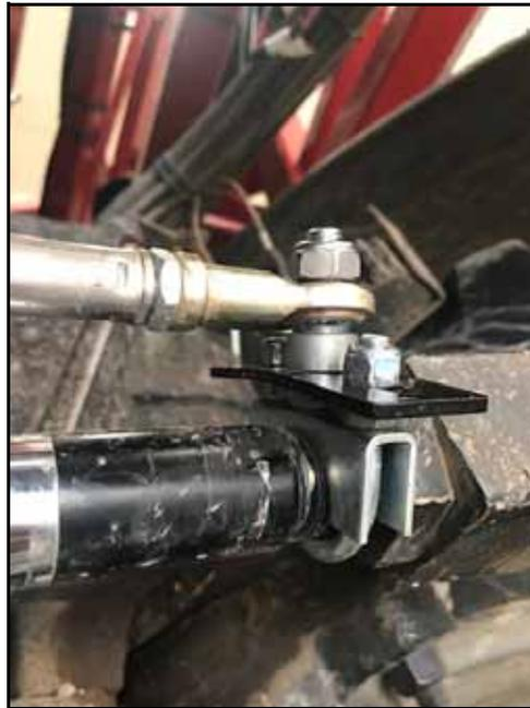
3. Remove the nuts and clamp from the 1-1/4" U-bolt clamp (P/N 435-3003-056).
