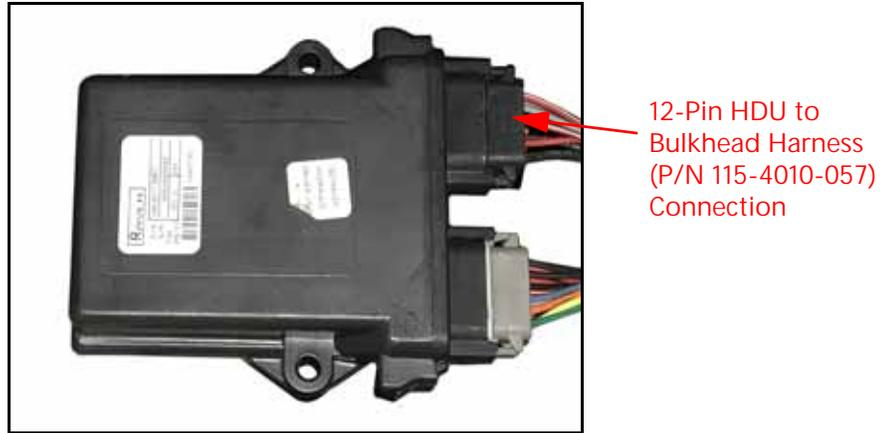
5. Connect the black 12-pin connector of the HDU to bulkhead harness cable (P/N 115-4010-057) to the mating port of the installed HDU (P/N 063-0173-887).
