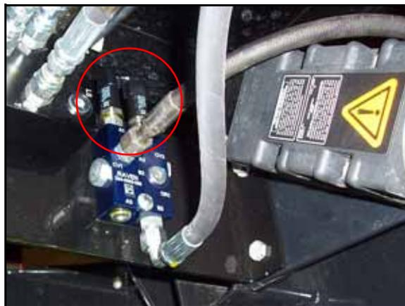
3. Install the PSI 1 and PSI 2 connectors on the pressure transducers installed in Ports A1 and B1 of the dual transducer pressure manifold (P/N 334-0003-085).
