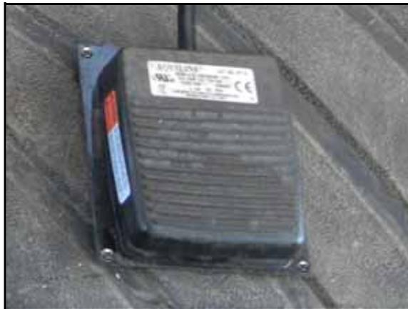
1. Select a suitable location for the foot switch (P/N 063-0173-470) to be installed.
