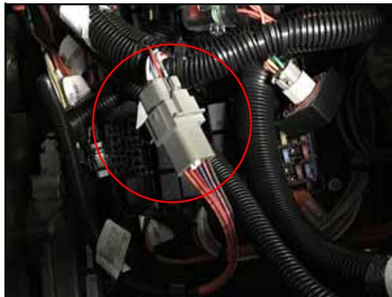
1. Connect the 8-pin CAB SWITCHES connector of the HDU harness cable (P/N 115-4010-185) to the mating female 8-pin connector of the HDU switch harness cable (P/N 115-4010-028).
