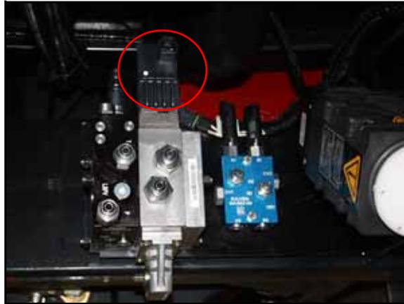
2. Connect the 4-pin VALVE connector to the open port of the SC1 hydraulic valve (P/N 334-0003-088).
