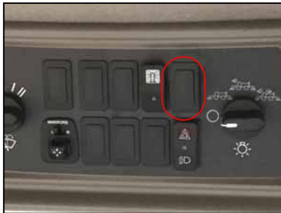
4. Locate an unused switch port of the machine's control console.
