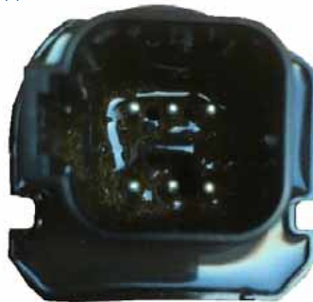
Cleaned Connector with Corrosion X HD Applied
