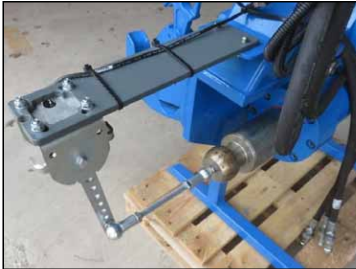
FIGURE 4. Top View of Angle Sensor Mounting
