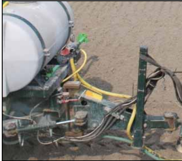
FIGURE 5. Angle Sensor Mounting on Side Shift Adapter Frame
