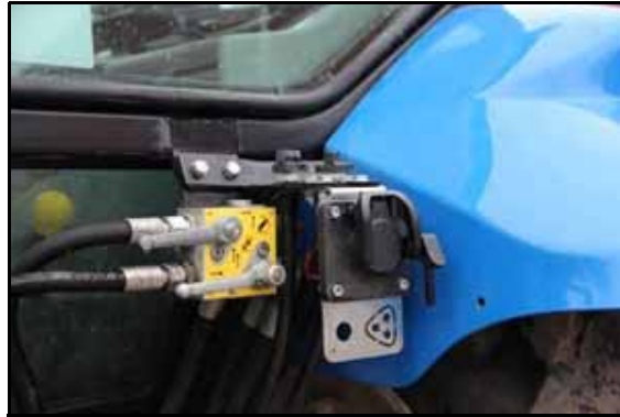
FIGURE 12. IBBC and IBBC Bracket with Antenna Connection
