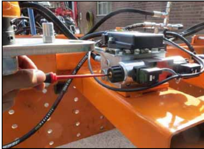
FIGURE 8. Proportional Valve Pin Used for Manual Steer
