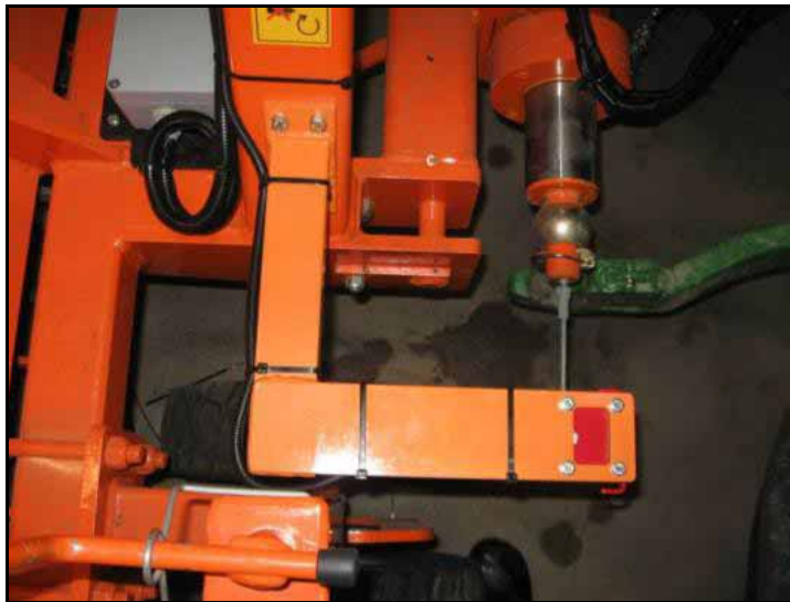
FIGURE 4. Top View of Angle Sensor Mounting
