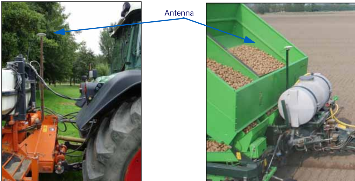
FIGURE 11. Examples of Antenna Mounting Positions
