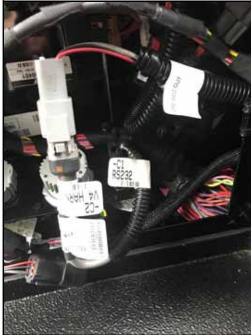
10. Connect the GPS REC OUT receptacle on the SC1 cable (P/N 115-0172-512) to the machine's existing X5088 INTERNAL GPS REC OUT plug.
