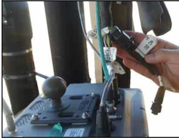
2. Plug the round ISO connector into the back of the Viper 4.
