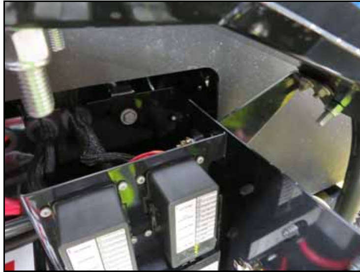
FIGURE 13. Ground Stud Location
