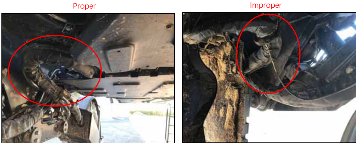
FIGURE 24. Proper and Improper Cable Routing
