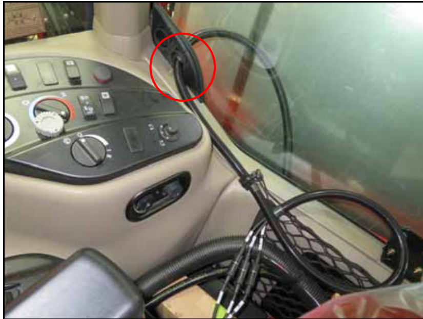
FIGURE 14. Cab Access Point
