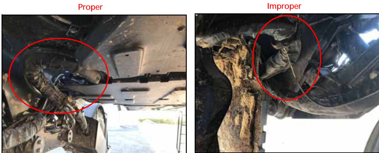
FIGURE 25. Proper and Improper Cable Routing
