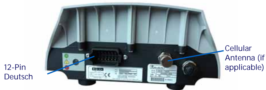
FIGURE 13. Cabling Connection on RS1 Unit
