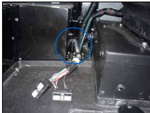
FIGURE 1. SmarTrax Node Harness to be Removed and Machine Access Panel
