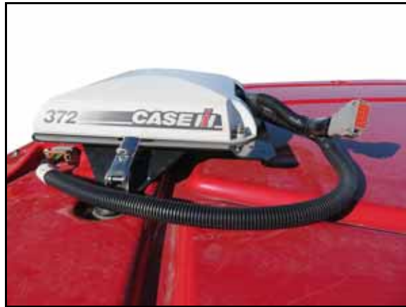
FIGURE 3. GPS Receiver Adapter Cable Installed
