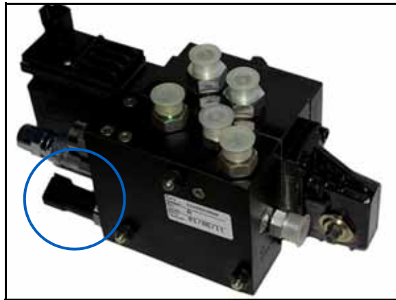
FIGURE 1. Pressure Transducer to be Removed
