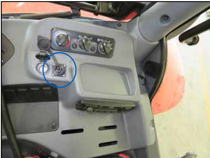
FIGURE 10. Power Terminal Location
