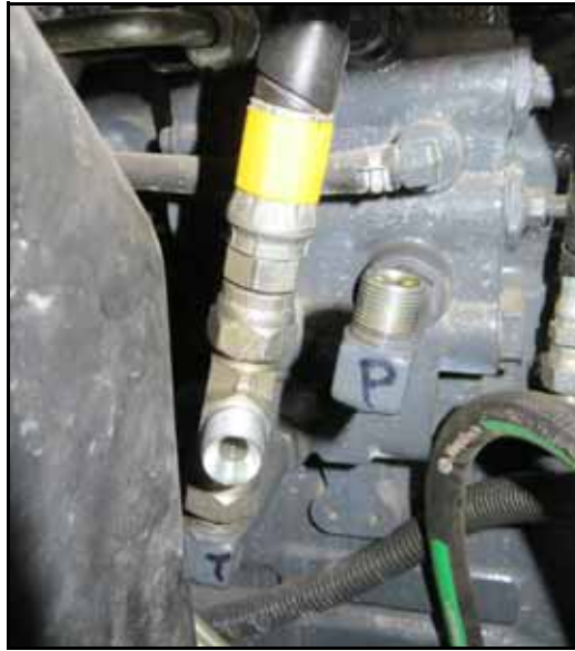
FIGURE 15. Tank Hose Connected with Run Tee
