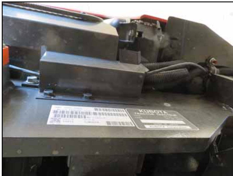
FIGURE 18. Wheel Angle Sensor Cable Routing
