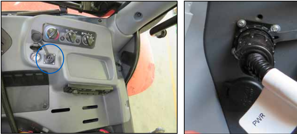
FIGURE 10. Power Terminal Location
