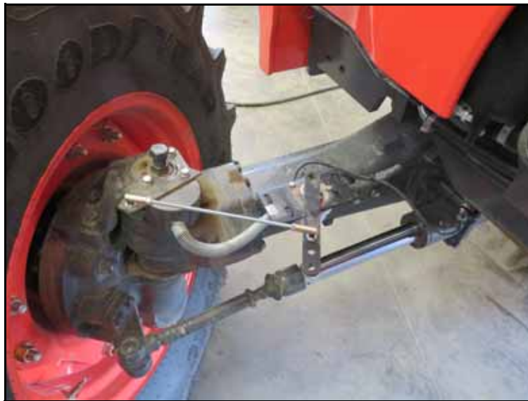
FIGURE 3. Bracket Attached to Wheel Hub
