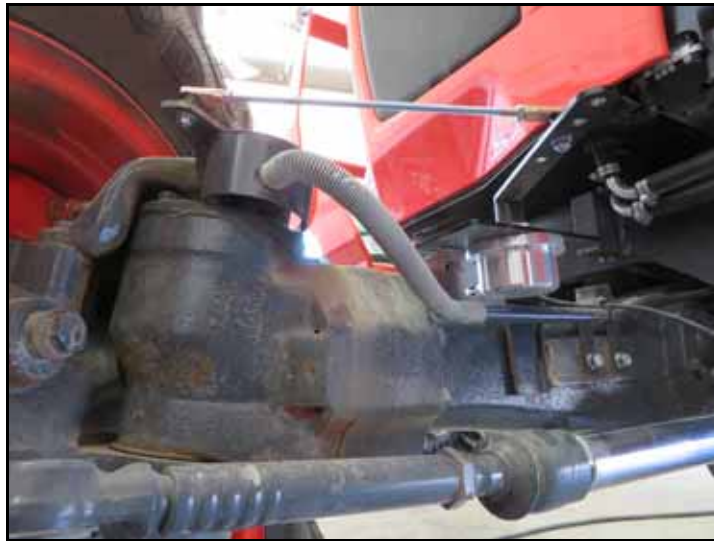
FIGURE 4. Wheel Angle Sensor Attached to Axle
