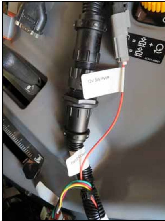
FIGURE 12. Switched Power and Field Computer Connections
