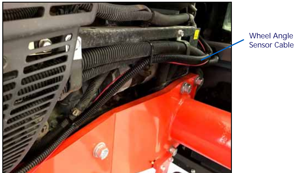
FIGURE 19. Wheel Angle Sensor Cable Routing
