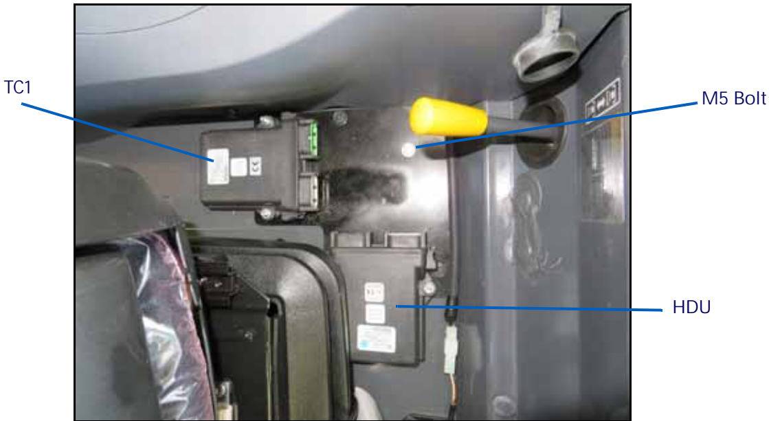
FIGURE 9. TC1 and HDU ECUs Installed
