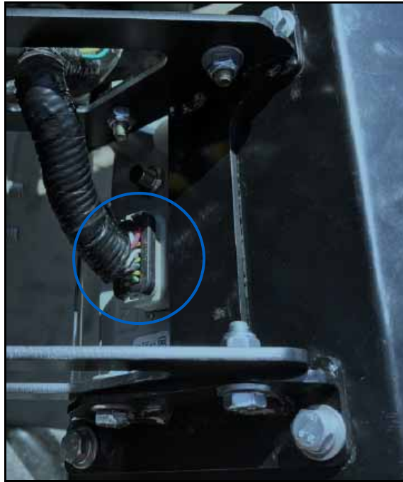
FIGURE 14. VSN Visual Guidance Camera Connection
