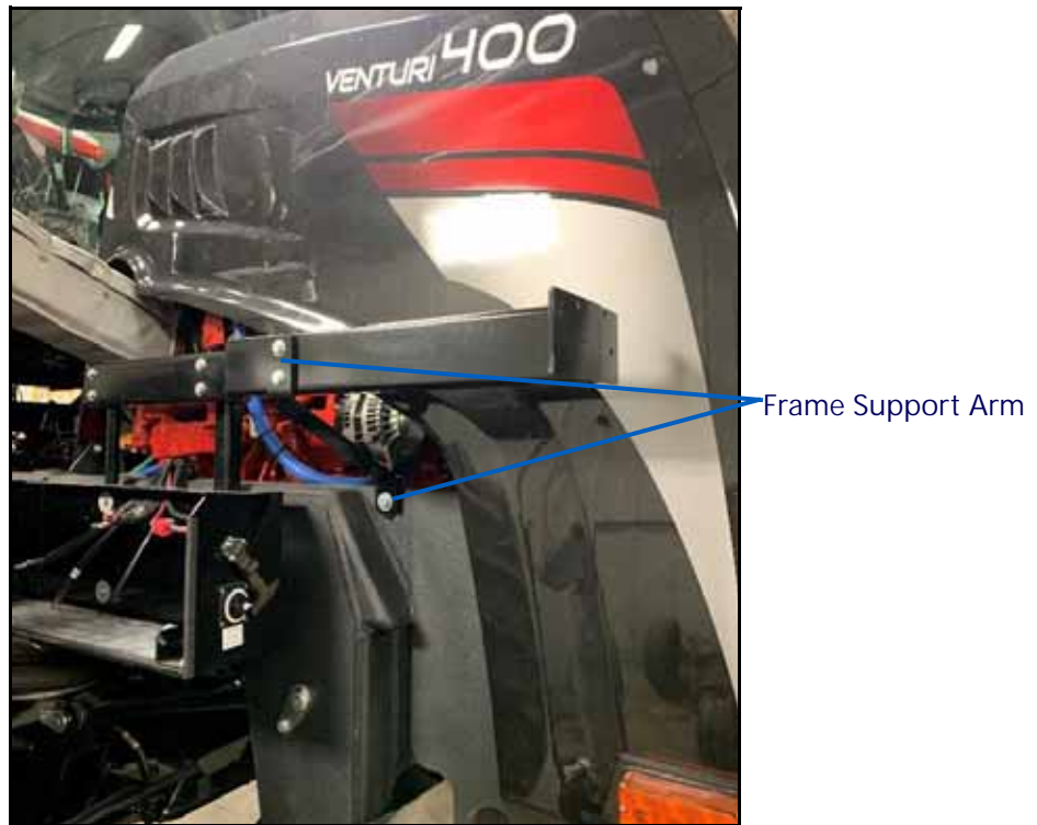
FIGURE 7. Installed Frame Support Arm
