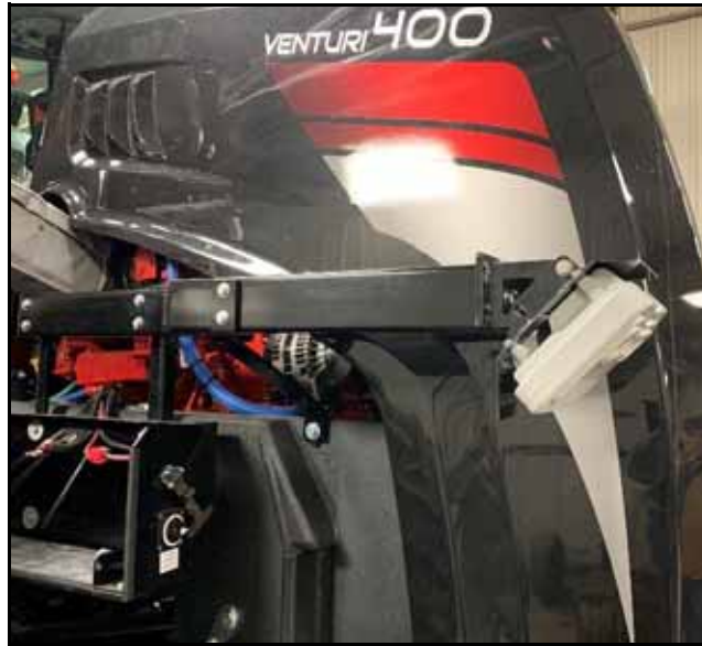
FIGURE 10. Installed Camera Assembly
