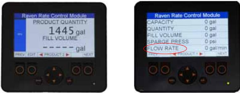
NOTE: The “FLOW RATE” reading indicates the rate of liquid product flowing into the tank.
