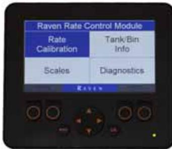
3. Press “ok” to enter the Rate Calibration screen.
