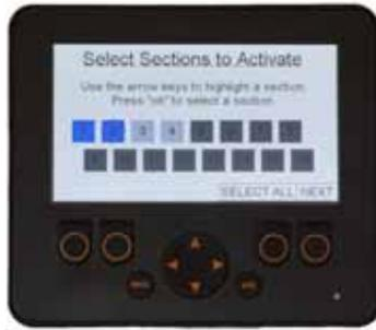
NOTE: The section selected must be turned on to press the “NEXT” button.
