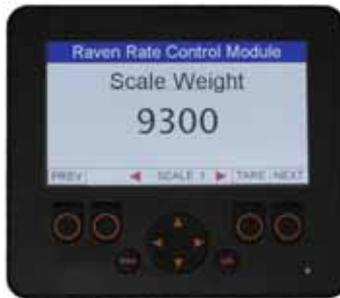
6. To zero out the product weight press the button directly below “ZERO”. Then press “ok” to accept that the tank will be zeroed out. Press CANCEL to cancel the operation.
