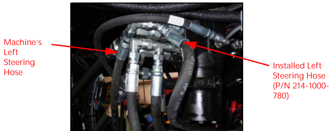
FIGURE 6. Left Steering Hose Installed on Steering Orbital
