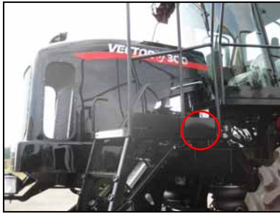
FIGURE 2. Steering Valve Mounting Location
