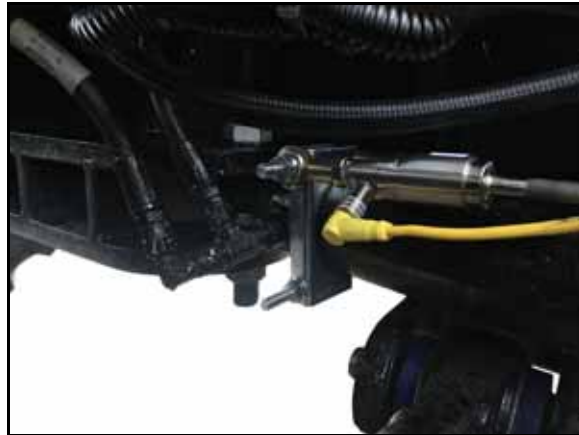
FIGURE 24. WAS Cable Connected to WAS
