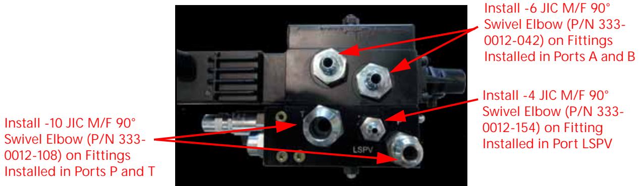
FIGURE 1. Fittings Installed in the Steering Valve
