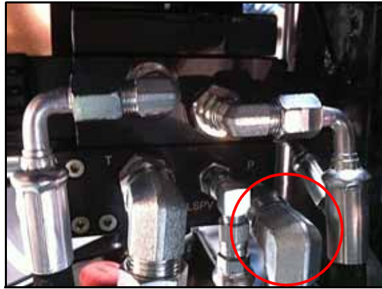
FIGURE 12. Pressure Hose Installed on Steering Valve
