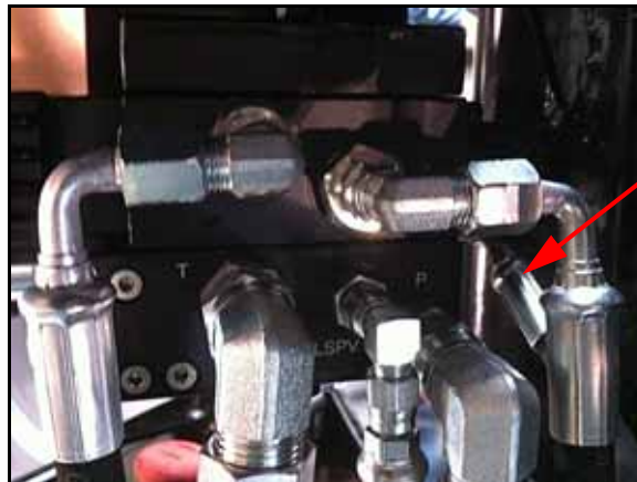
FIGURE 17. LS STEER Connection on Steering Valve
