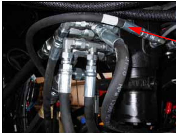
FIGURE 16. Load Sense Hose Installed on Steering Orbital
