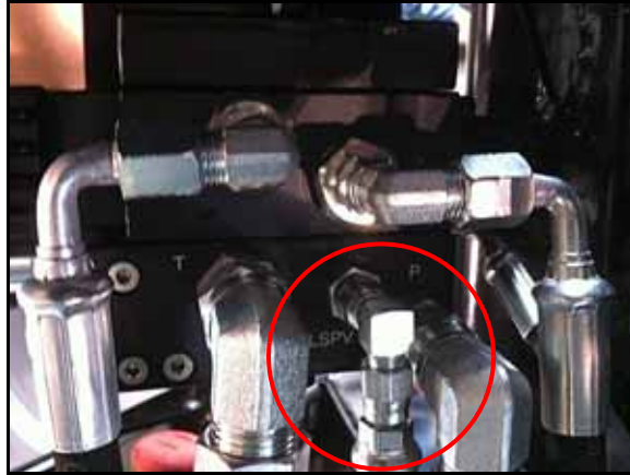
FIGURE 15. LSPV Connection on Steering Valve
