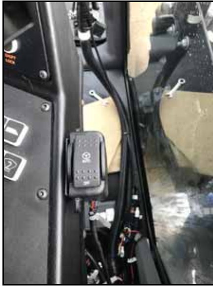
FIGURE 14. 2-Pin Engage to SmarTrax Cable
