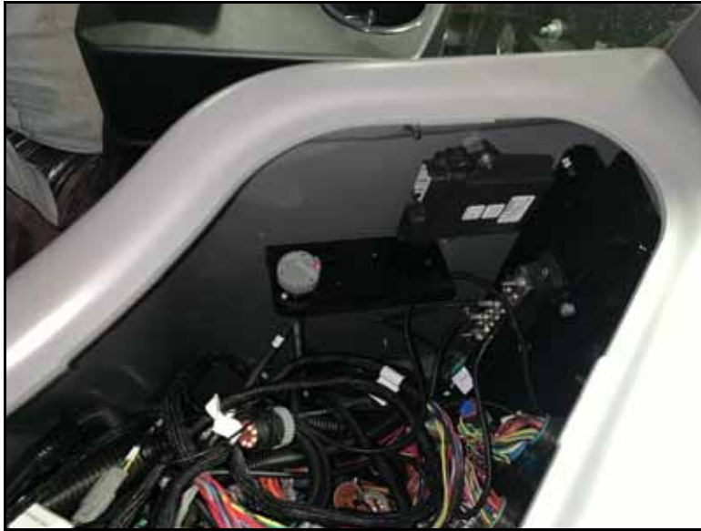
FIGURE 7. ECU Mounting Orientation
