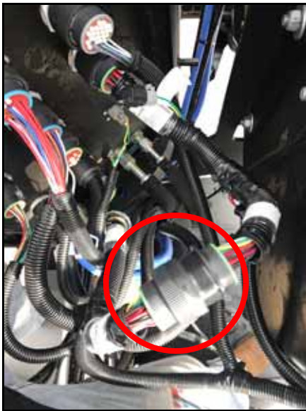
FIGURE 18. RS1 Connected to Machine's Mating Connector
