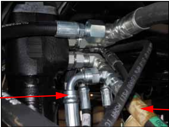
FIGURE 11. Pressure Hose Installed on Steering Orbital
