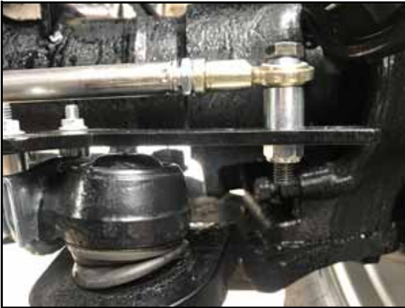
FIGURE 5. WAS Rod Mounting Bracket Installation
