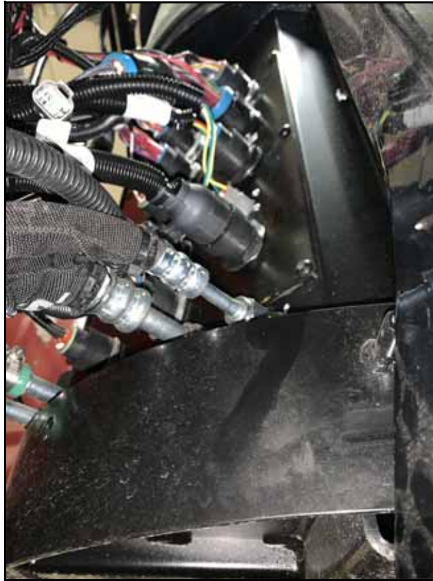
FIGURE 22. Valve Cable Connected to Bulkhead
