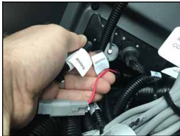
FIGURE 14. 2-Pin Engage to SmarTrax Cable
