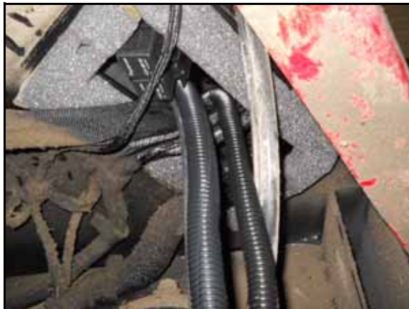
FIGURE 11. Valve Harness Routed Outside the Cab
