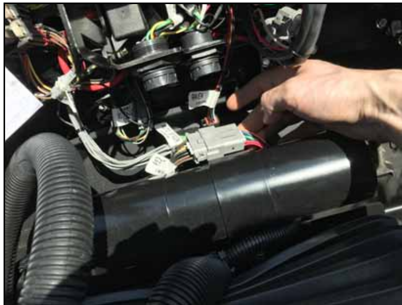
FIGURE 9. Operator Presence Tee Connection with Seat Connector
