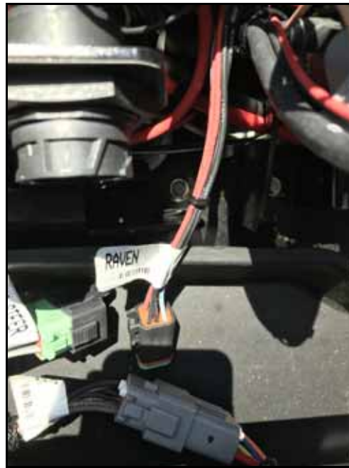
FIGURE 8. Raven Connector Located in Compartment Behind the Seat
