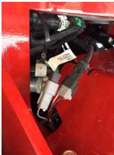
FIGURE 13. WAS Connection on Articulated Machine
