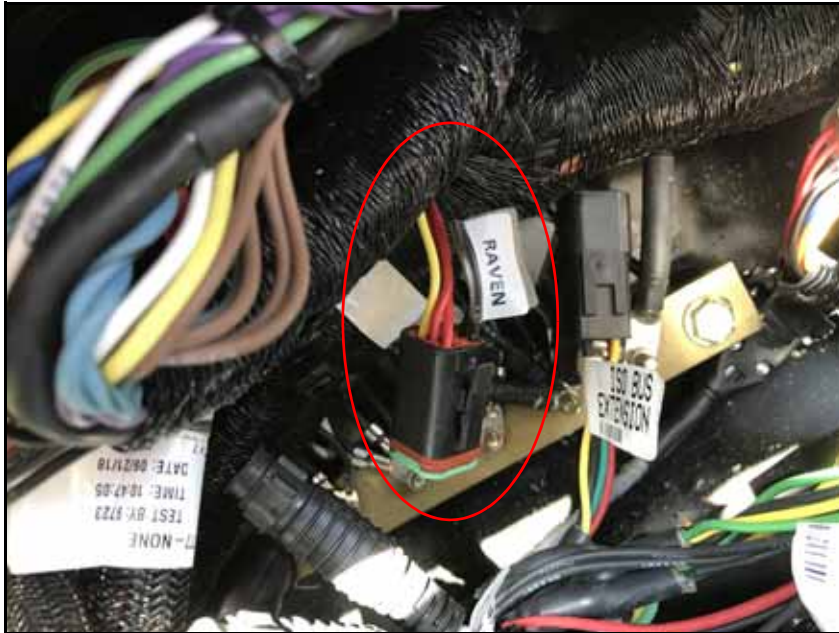
FIGURE 4. 6-Pin Deutsch Connector on Node Harness
