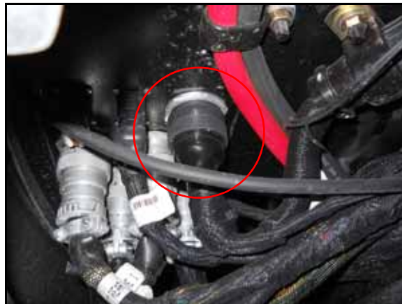
FIGURE 10. Valve Harness Secured to Bulkhead
