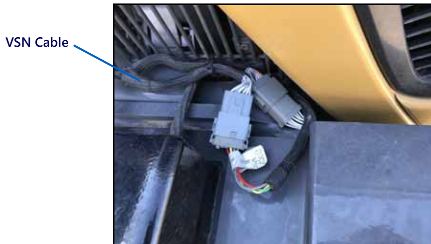
FIGURE 14. Switched Power Tee Connection
