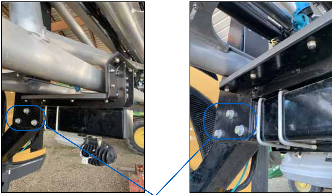
FIGURE 2. Cradle Bracket Hardware for Millennium Boom Configurations
