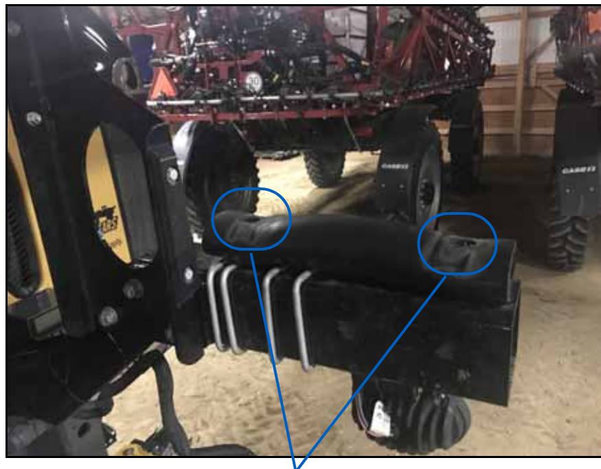
FIGURE 1. Cradle Frame Cushion Hardware
