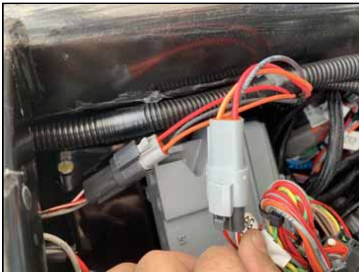
FIGURE 12. Power Tee Connection
