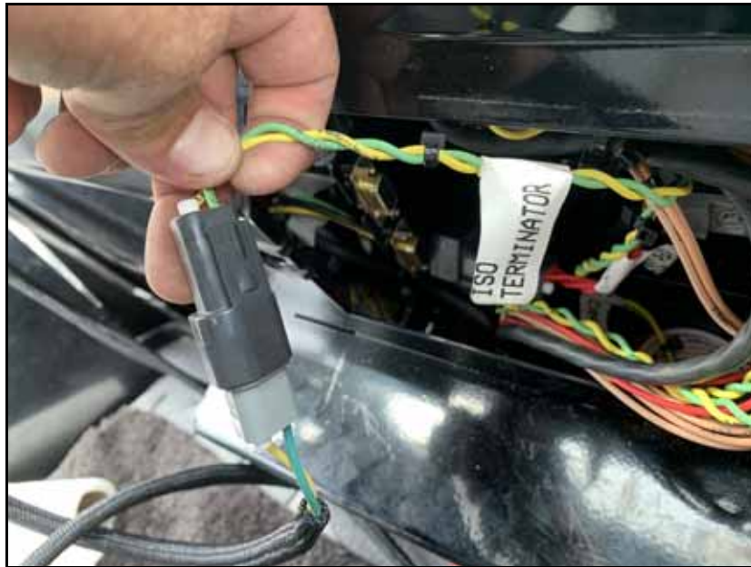
FIGURE 13. ISO Terminator Connection
