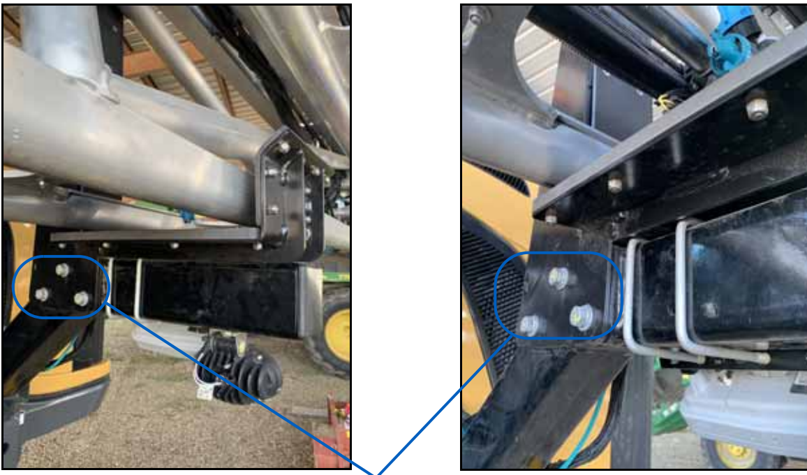
FIGURE 2. Cradle Bracket Hardware for Millennium Boom Configurations
