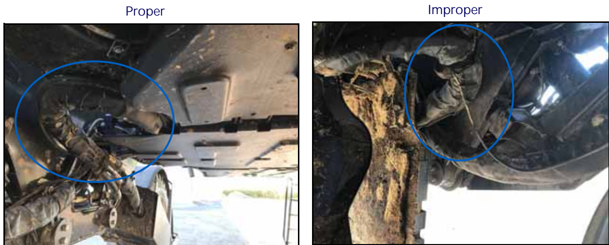
FIGURE 20. Proper and Improper Cable Routing
