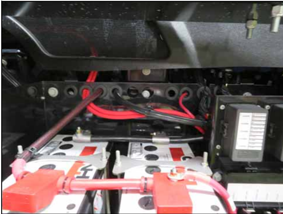
FIGURE 9. Power Connection Routing
