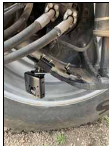
Right Bracket Installed
