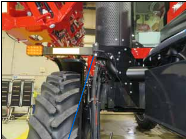
M8 Hardware to be removed
