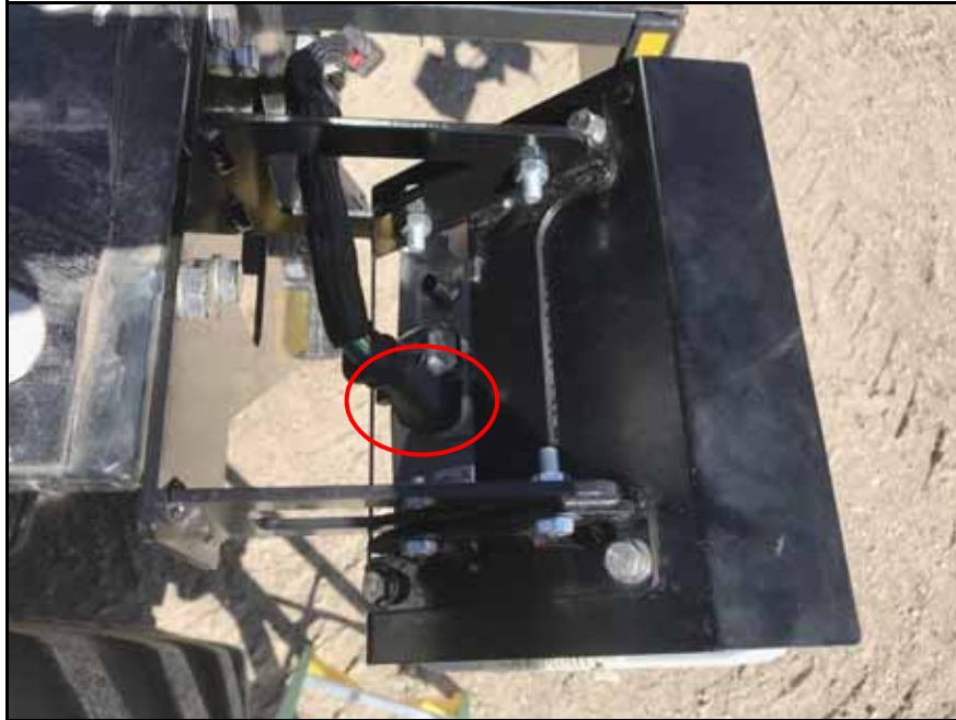
FIGURE 9. VSN Camera Connection
