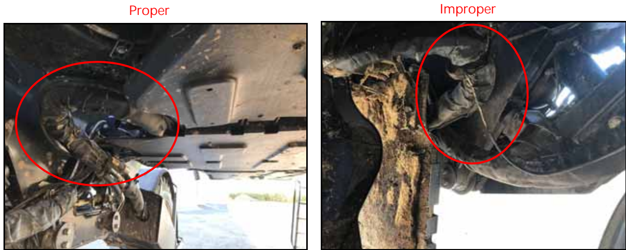
FIGURE 21. Proper and Improper Cable Routing
