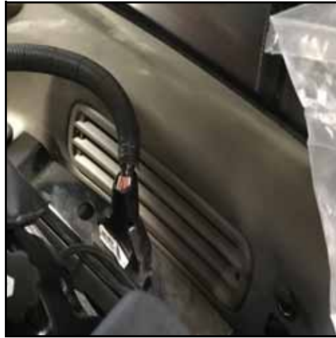
FIGURE 13. Remove Vent Cover to Access Connectors
