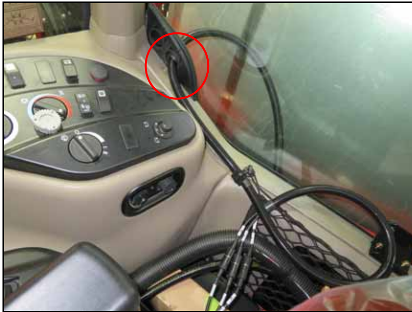
FIGURE 15. Cab Access Point
