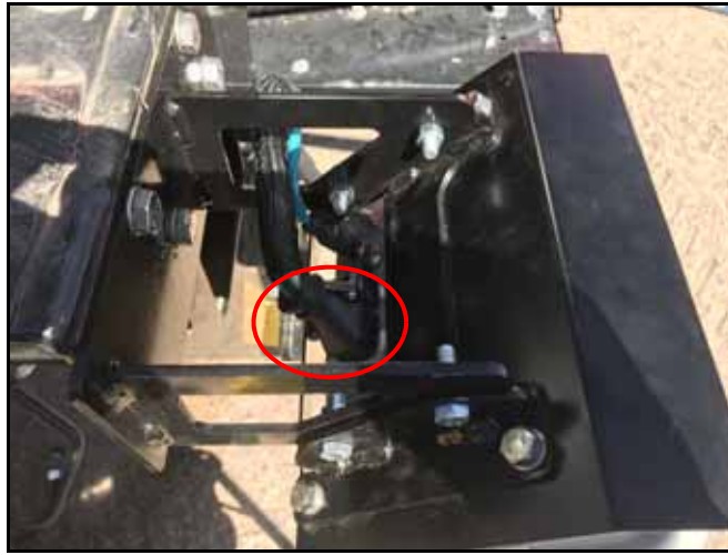
FIGURE 11. VSN Camera Connection
