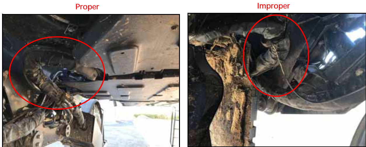
FIGURE 24. Proper and Improper Cable Routing
