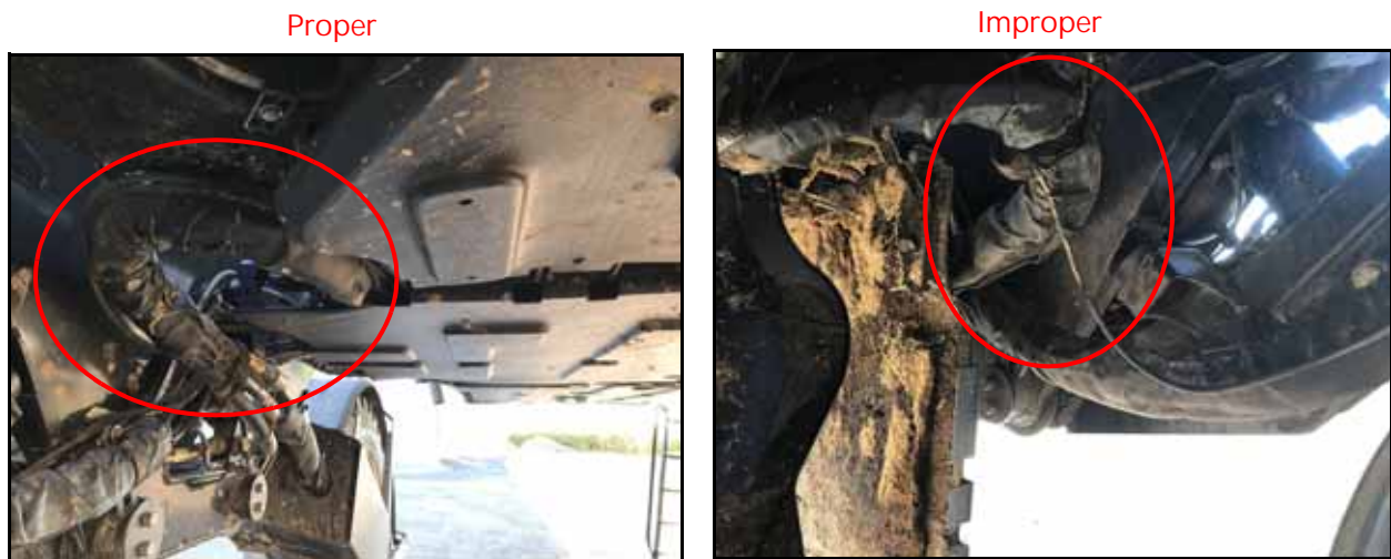
FIGURE 24. Proper and Improper Cable Routing
