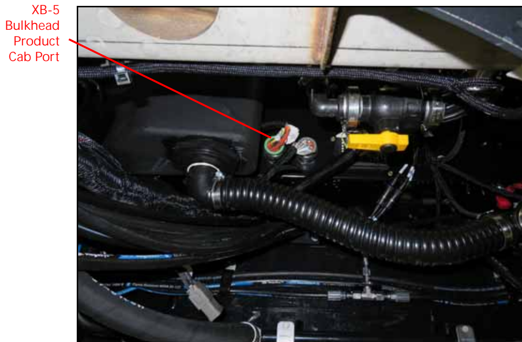
FIGURE 10. XB-5 Bulkhead Product Cab Connection
