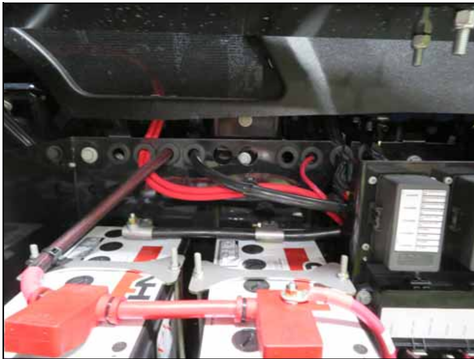
FIGURE 12. Power Connection Routing
