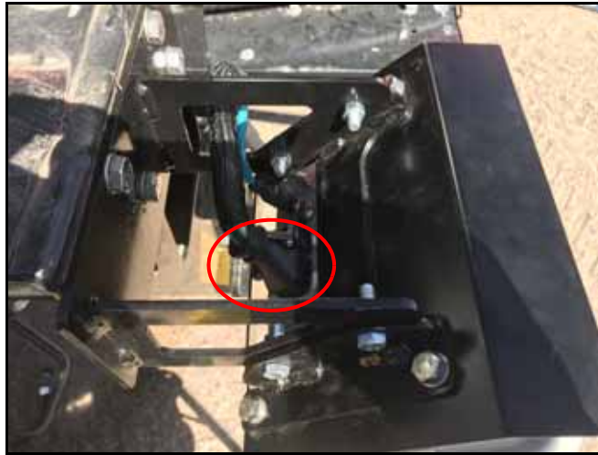
FIGURE 11. VSN Camera Connection
