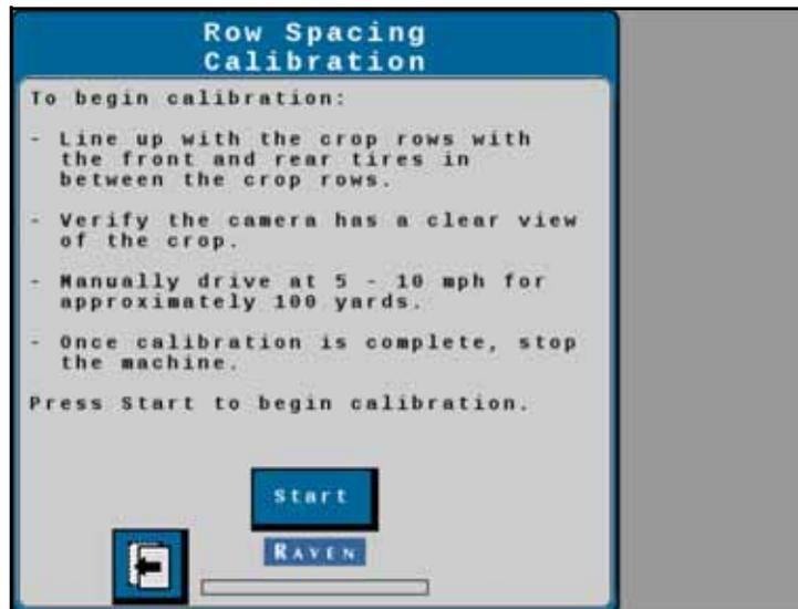
6. Drive slowly down the row while steering the machine manually. Drive at a speed of 5 to 10 mph [8.5 to 16 km/h]. After approximately 100 yards [91 m], the calibration process will be complete.
