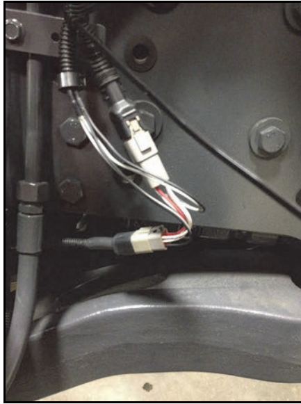
FIGURE 14. WAS Tee to Valve Harness Connection
