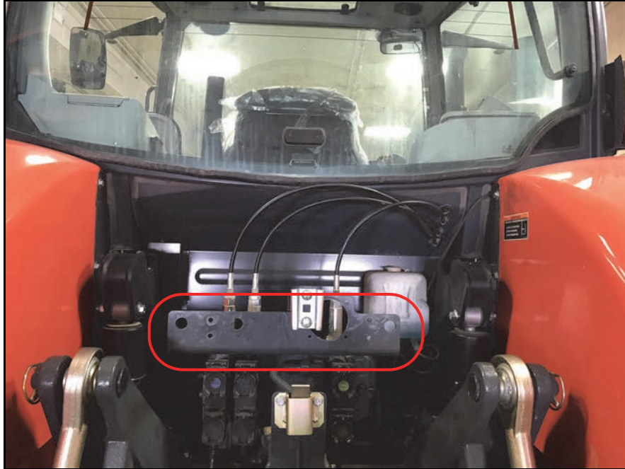
FIGURE 3. Steering Valve Assembly Mounting Location
