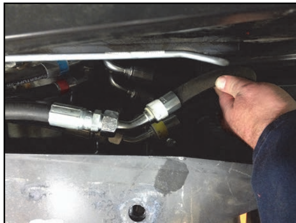
FIGURE 12. Hydraulic Hose Installed on Left Steering Hose
