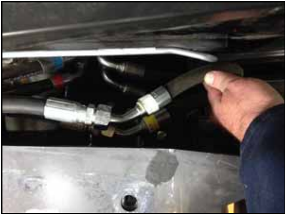
FIGURE 17. Hydraulic Hose Installed on Right Steering Hose
