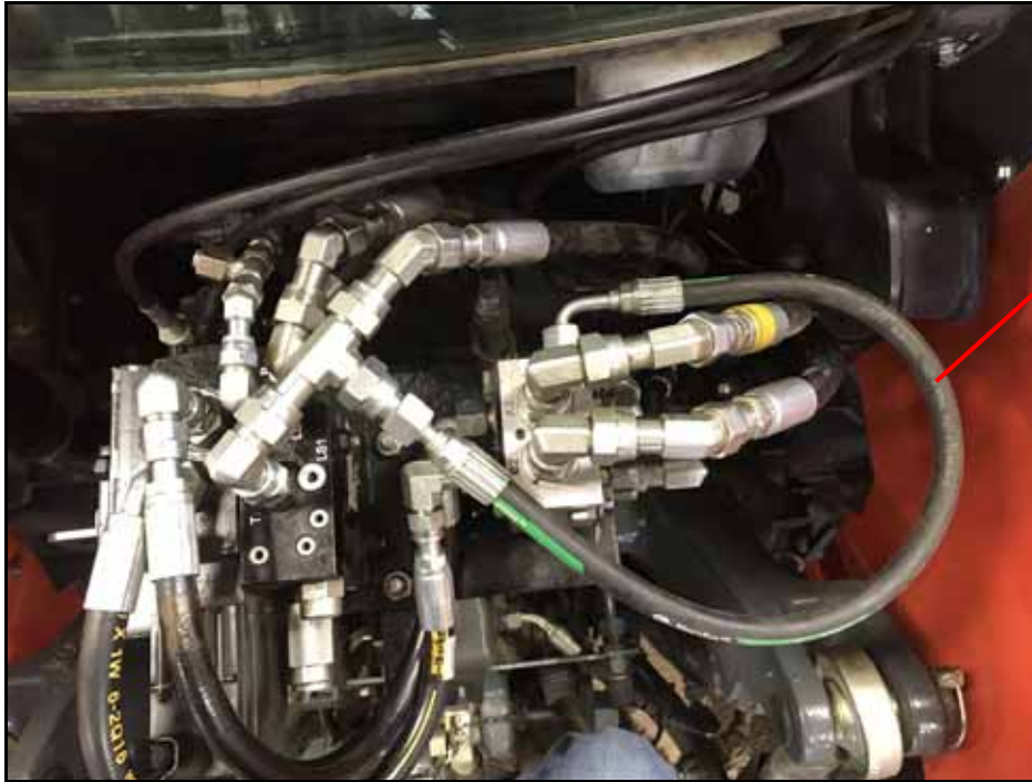
FIGURE 33. Tank Relief Hose Installed
