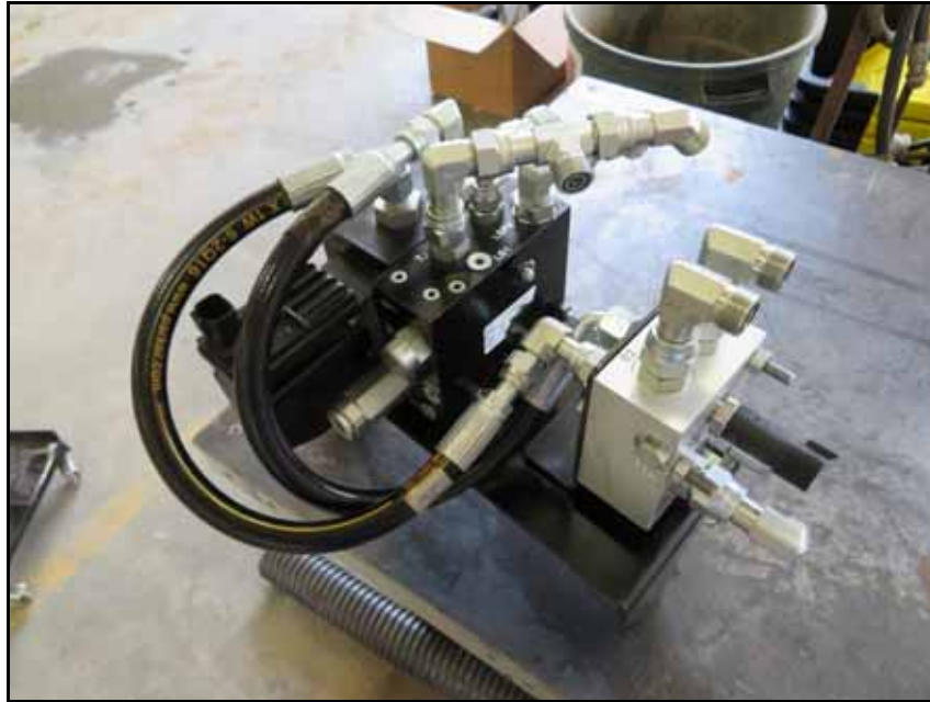
FIGURE 19. Right Steering Hose Installed on the Hydraulic Steering and Dual POCI Valve
