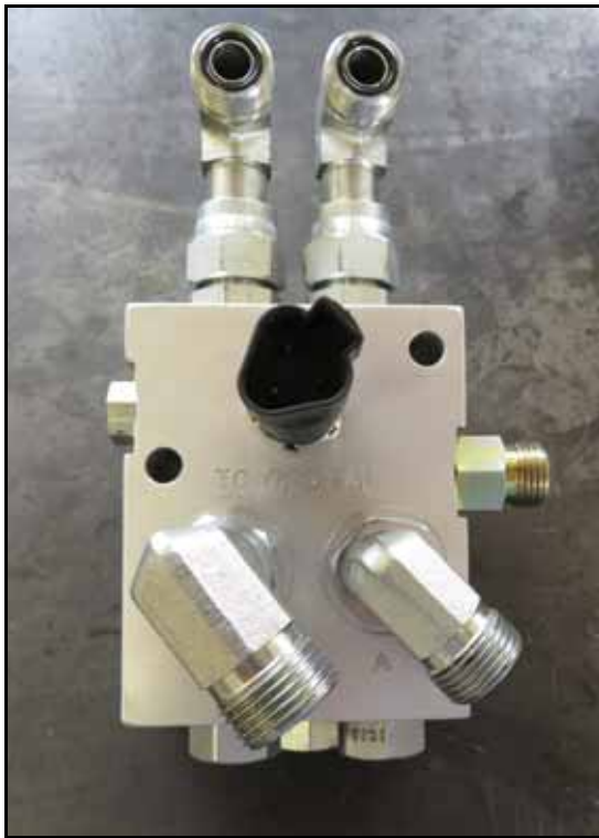
FIGURE 2. Fittings Installed on Dual POCI Valve
