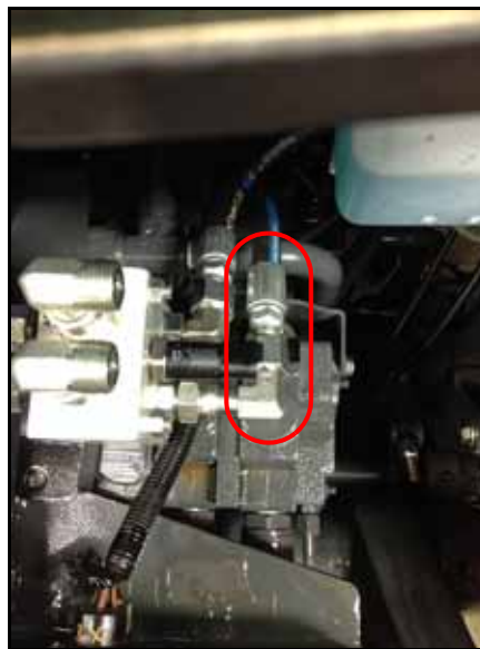
FIGURE 16. Hydraulic Hose Installed on Dual POCI Valve Port B
