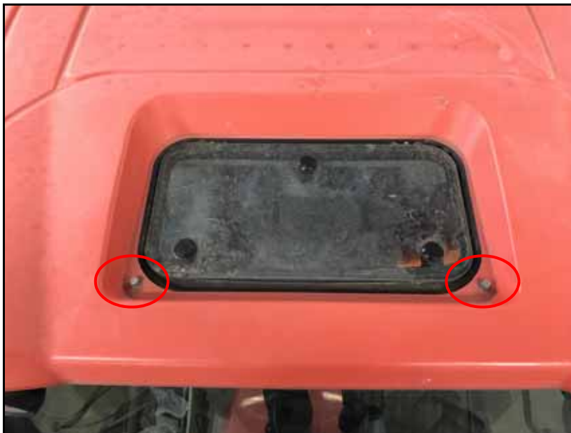
FIGURE 14. Rooftop Mounting Location
