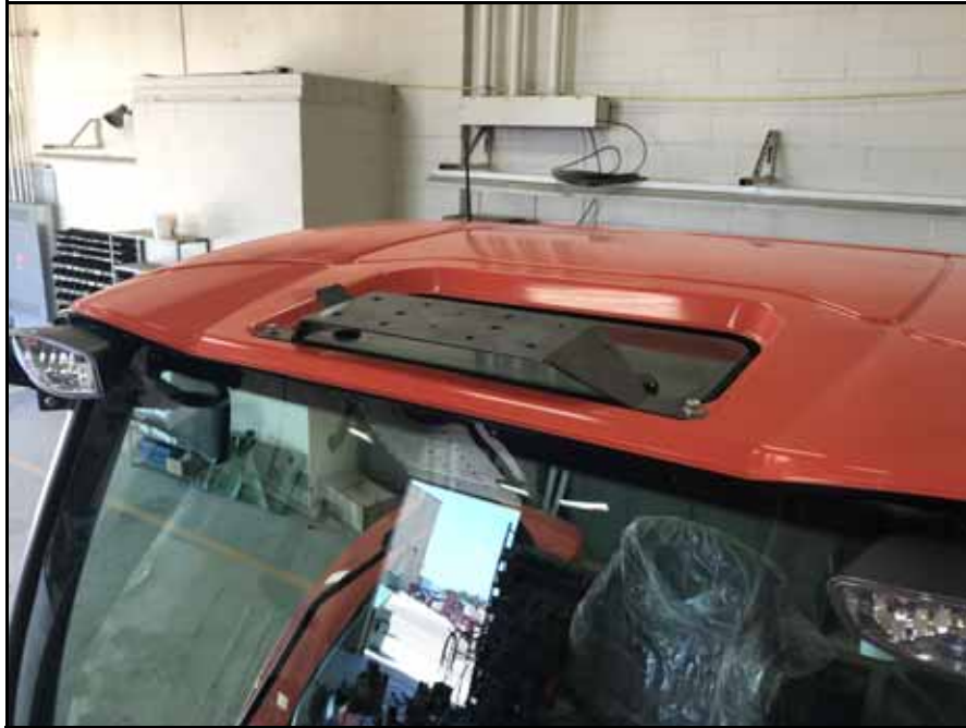
FIGURE 15. Mounting Bracket Installed
