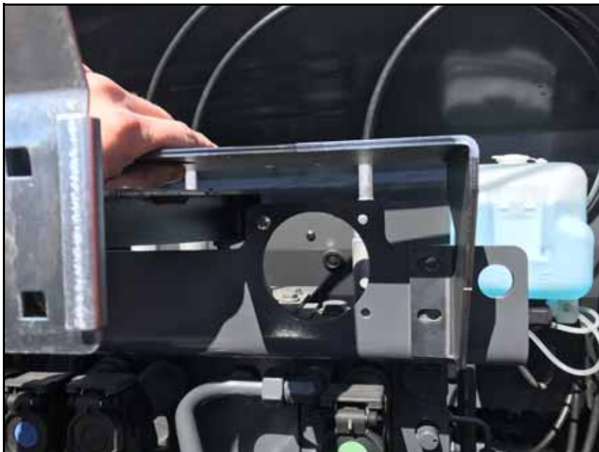
FIGURE 4. Valve Mounting Base Bracket Installed
