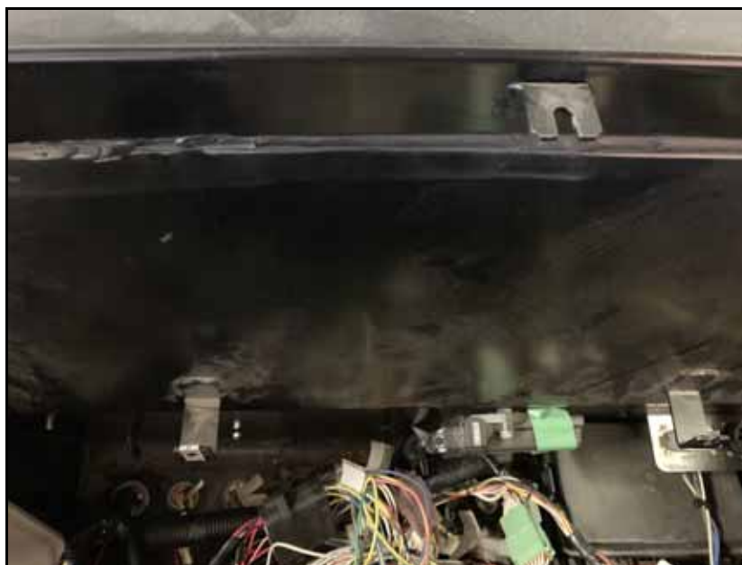
FIGURE 4. Access Panel to be Removed
