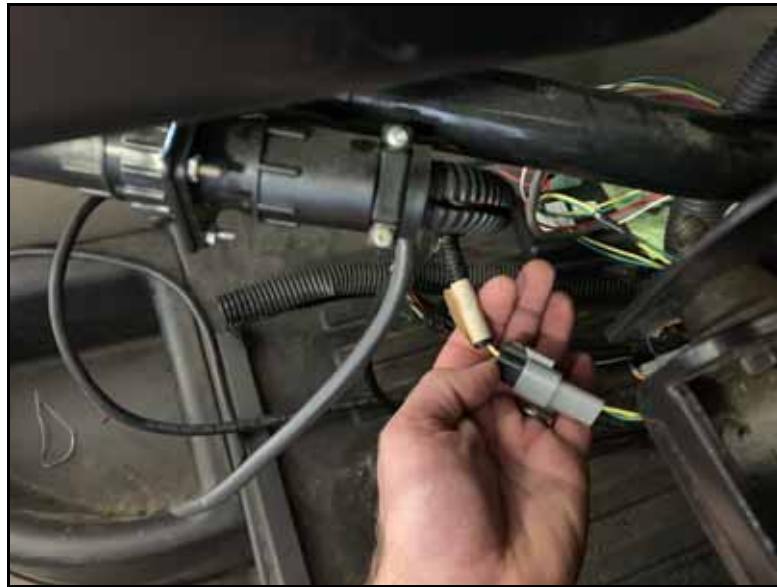
FIGURE 8. HDU Cable Connected
