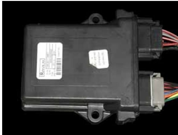
FIGURE 12. HDU Harness Cable Installed on HDU
