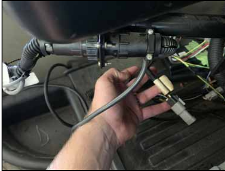
FIGURE 7. Existing CAN Terminator
