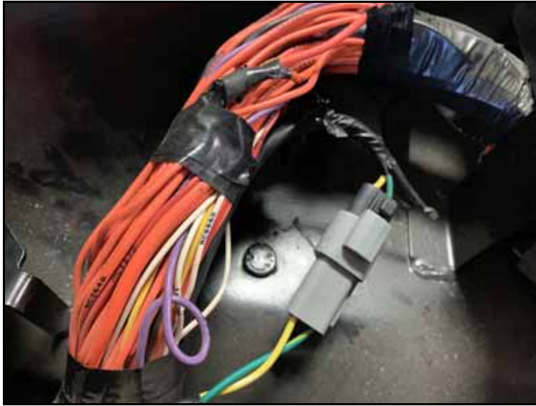
FIGURE 12. HDU Harness Cable Installed on HDU
