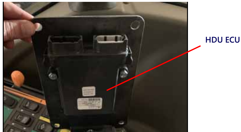
FIGURE 13. HDU Installed on HDU Mounting Bracket
