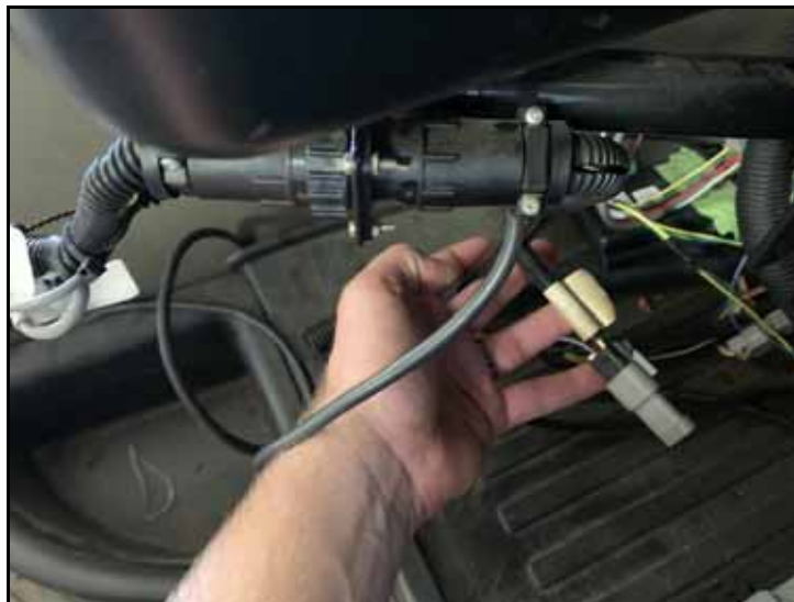
FIGURE 6. Existing CAN Terminator
