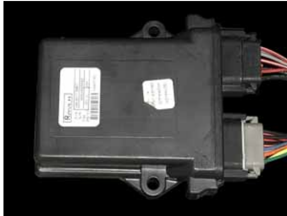
FIGURE 11. HDU Harness Cable Installed on HDU
