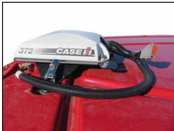
FIGURE 2. GPS Receiver Adapter Cable Installed
