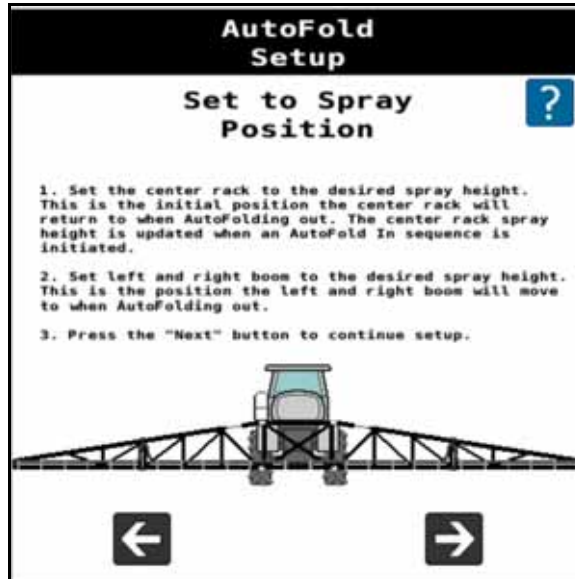
FIGURE 6. Vertical Center Sensor Calibration - Set to Spray Position
