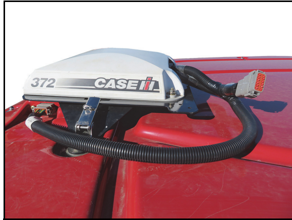
FIGURE 5. GPS Receiver Adapter Cable Connection
