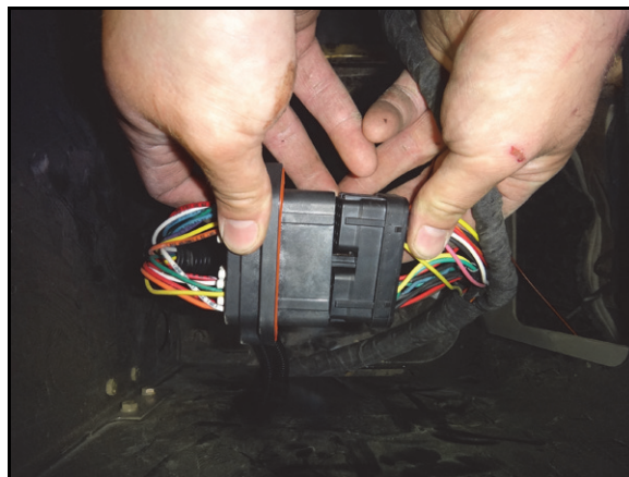
FIGURE 6. ECU Harness Connected to Machine Harness
