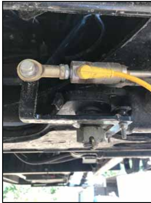
FIGURE 11. Small WAS Mounting Bracket Installed on Rod-End of Steering Cylinder
