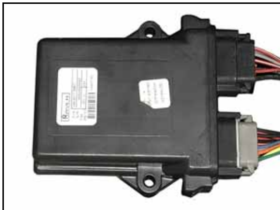
FIGURE 6. HDU Harness Cable Installed on HDU
