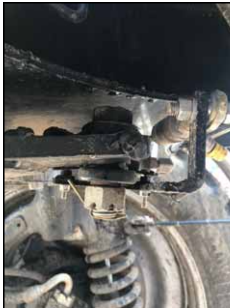
FIGURE 13. Base-End of WAS Installed on Base-End of Steering Cylinder
