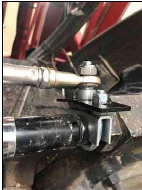
FIGURE 11. Small WAS Mounting Bracket Installed on Rod-End of Steering Cylinder
