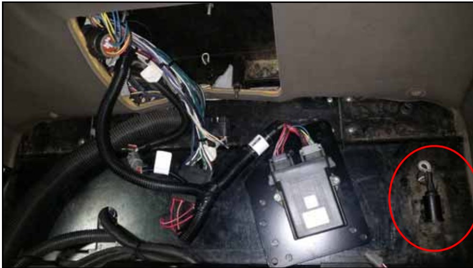
FIGURE 6. SC1 Node Mounting Location
