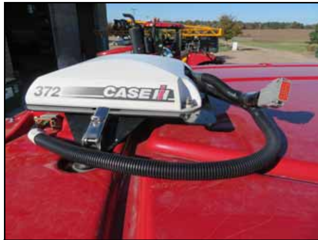
FIGURE 1. GPS Receiver Adapter Cable Connection
