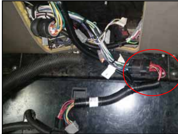
FIGURE 5. HDU Harness Cable Installed on HDU
