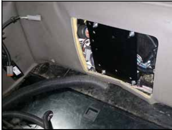
FIGURE 9. HDU Mounting Bracket Installed
