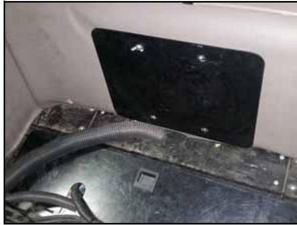
FIGURE 2. Access Panel to be Removed
