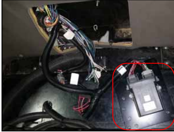
FIGURE 8. HDU Installed on HDU Mounting Bracket
