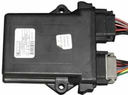
FIGURE 5. HDU Harness Cable Installed on HDU
