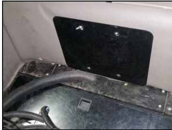
FIGURE 10. Access Panel to be Removed
