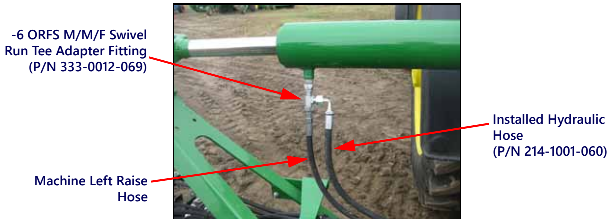
FIGURE 17. Raise Hose Installed on Left Tilt Cylinder
