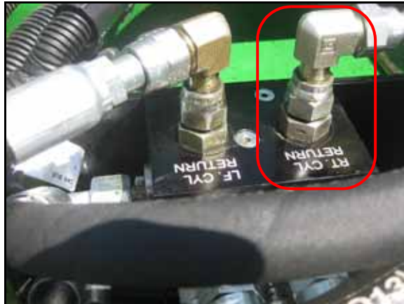
FIGURE 27. Right Down Hose Installed on AutoBoom Valve
