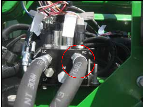
FIGURE 21. Right Raise Hose Installed on AutoBoom Valve
