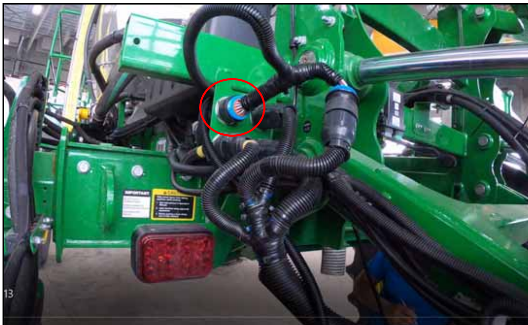
FIGURE 10. AutoBoom Harness Cable Installed
