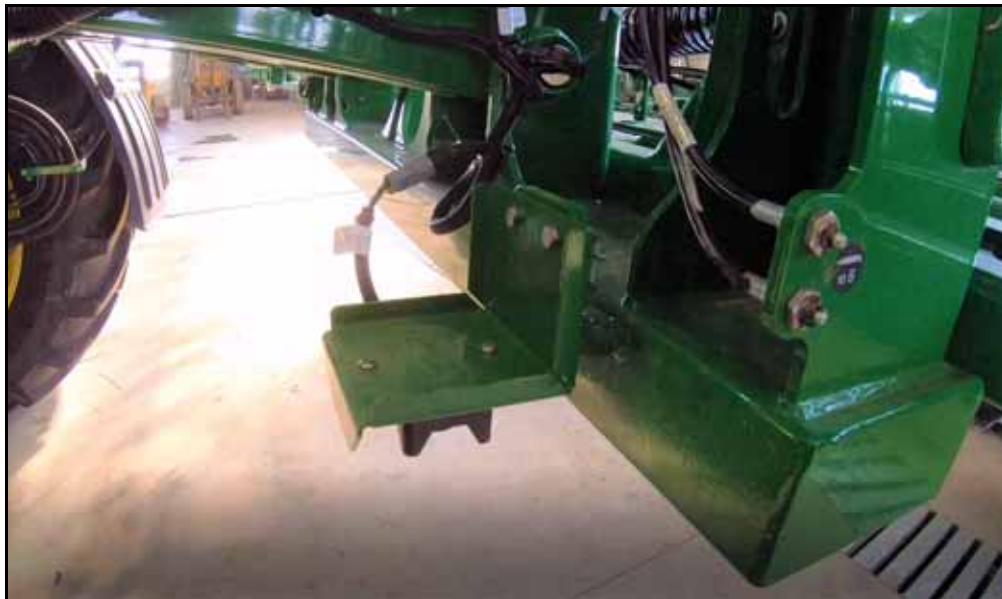
FIGURE 4. Center Sensor Installed
