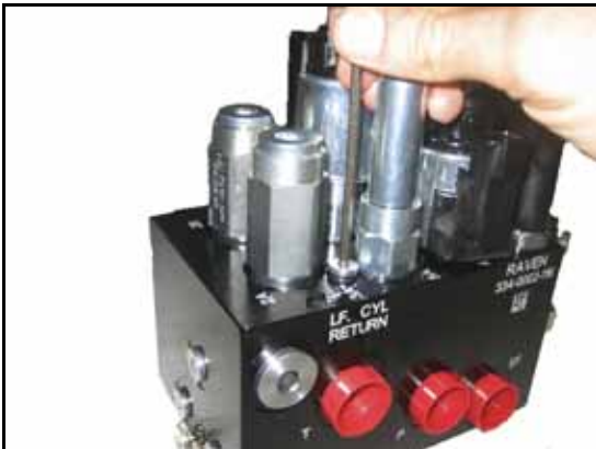
FIGURE 5. Port Plug Reinstalled on the AutoBoom Valve
