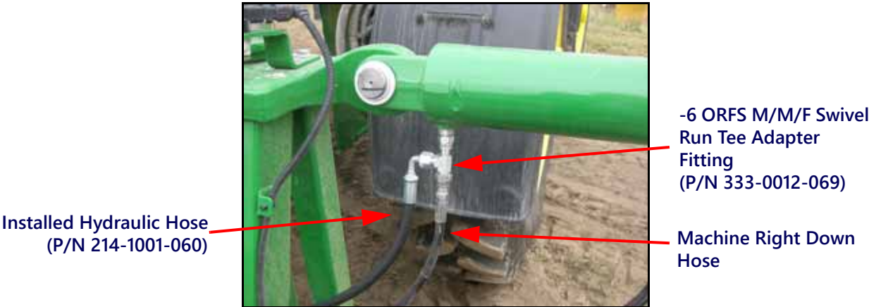
FIGURE 26. Down Hose Installed on Right Tilt Cylinder
