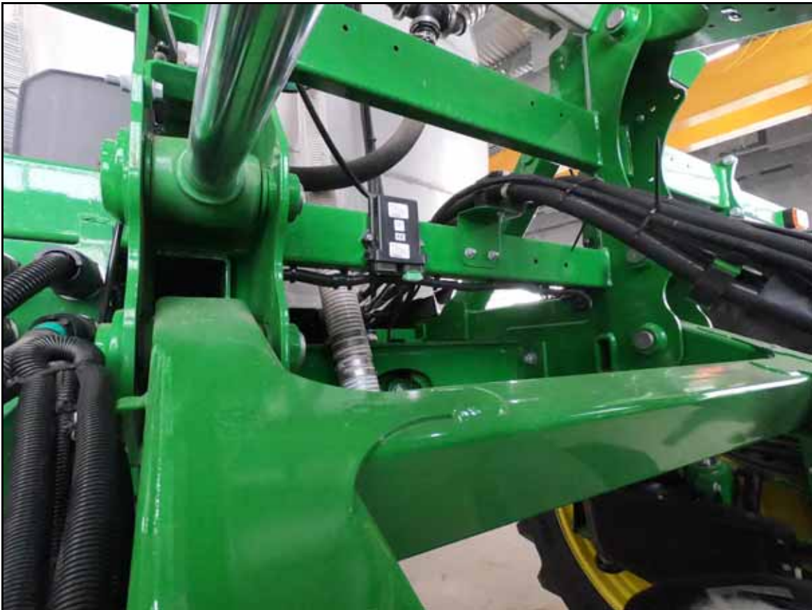
FIGURE 1. Installed AutoBoom XRT Node
