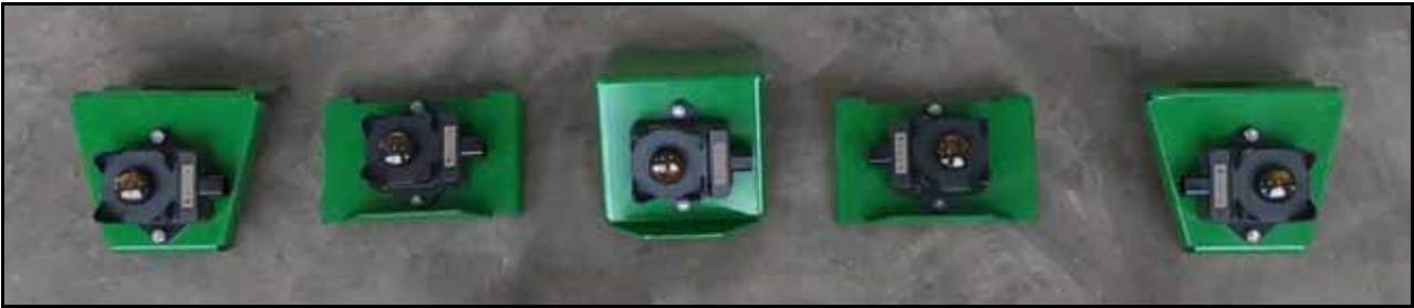
FIGURE 1. Sensor Installed on Mounting Bracket
