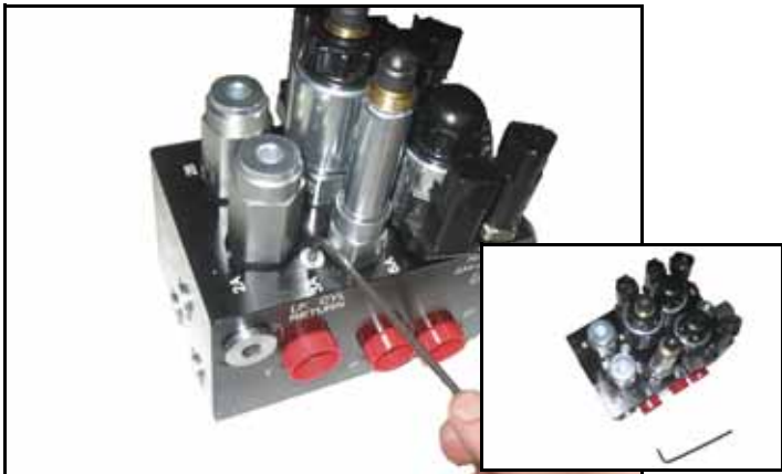
FIGURE 3. Port Plugs Removed from the AutoBoom Valve
