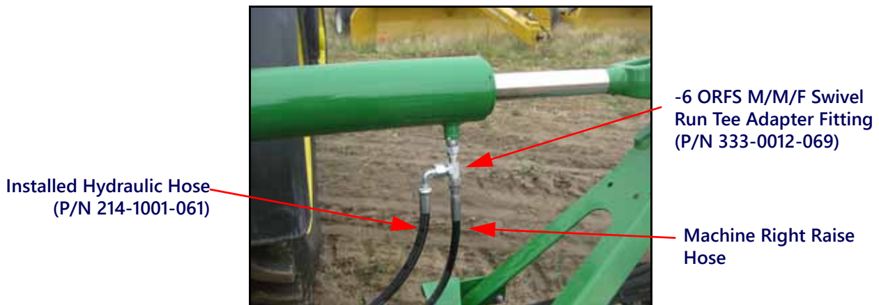
FIGURE 20. Raise Hose Installed on Right Tilt Cylinder
