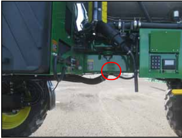
FIGURE 13. Load Sense Jam Valve
