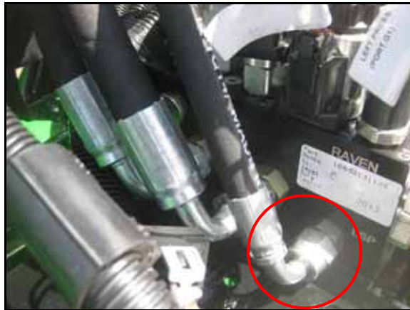
FIGURE 30. Load Sense Hose Installed on AutoBoom Valve
