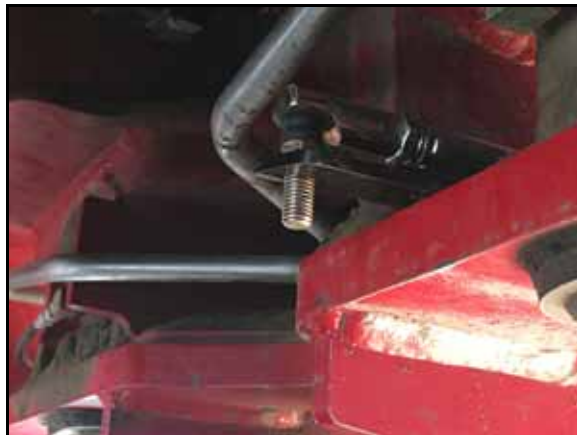
FIGURE 11. Rod-End of Sensor Installed
