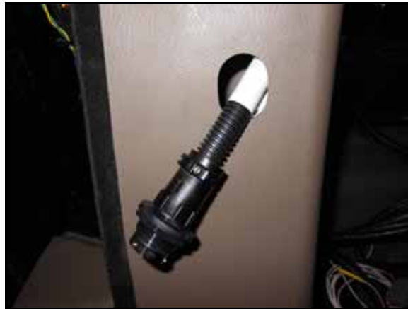
FIGURE 20. ISO Bus Display Adapter Harness Routed Through Post Cover
