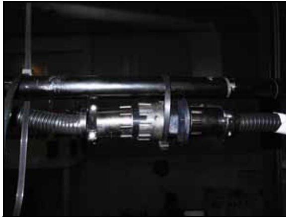
FIGURE 22. ISO Bus Adapter Harness Connected to CR7 or Viper 4 Harness
