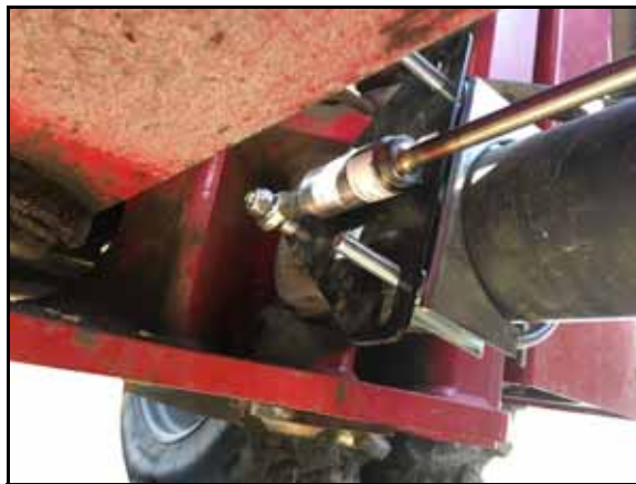
FIGURE 5. Base-End of Sensor Installed
