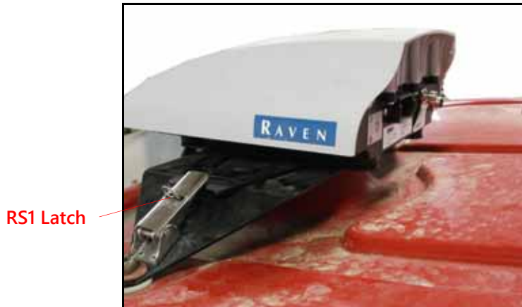
FIGURE 3. Installed RS1 Unit
