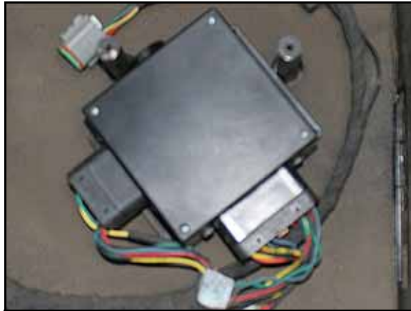
FIGURE 9. Case Cable Connected to the Case Interface Box
