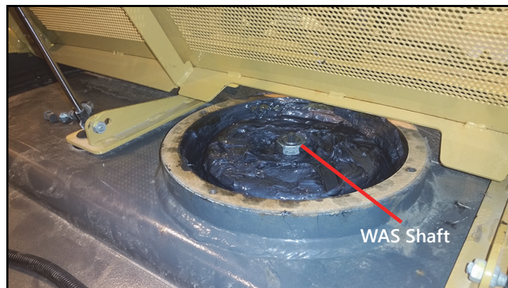
FIGURE 2. Installed WAS Shaft
